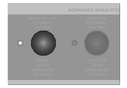
This means that if, for example, you edit LFO 3 in the LFO section, then the parameters Rate, Shape and Keyfollow are directly accessible as is the case with LFO 2. However, LFO 3 does not feature the Contour parameter. Consequently, the LED of the Contour knob will not light up since the knob serves no function in this situation.
