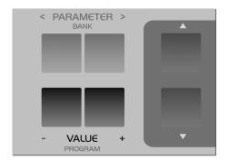
Use the *UP* or *DOWN* buttons to activate the filter section FILT. The second encoder knob in this row is labeled CUTOFF (not to be confused with CUTOFF 2!). Rotate the encoder to the left and right and note how the sound becomes muddier and clearer in response to the direction in which you turn the encoder. (To ensure this effect and the following aural experiments are most pronounced, adjust the amplifier envelope so that the Virus generates a constant level while you hold a key down).
