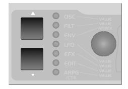
Take a look at the display of the Virus to gain an impression of the difference between these two values. It shows two numeric values when you dial a encoder: at the left you can see the value stored in the sound program and at the right, the numeric equivalent to the value determined by the current position of the encoder
