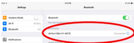
The AirTurn BT-106 should appear under the list of Bluetooth devices. Follow prompts for adding a Bluetooth device if your tablet or computer requires it. Tap or click on the AirTurn BT-106 serial number to connect. If your tablet or computer prompts you to confirm a passcode, select "OK" or "YES" to finish the pairing.
