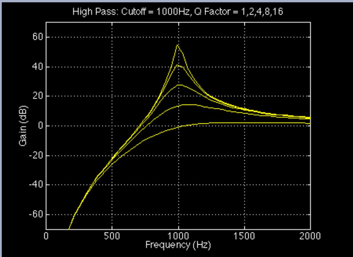
*High pass filter response curves for different values of  $Q$ . A low  $Q$  filter has a smooth roll off. A high  $Q$  filter has a resonance peak before the cutoff frequency.*
