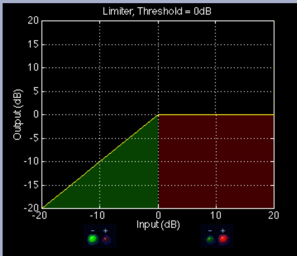
*As signal rises toward zero dB, no limiting is applied. Any signal that exceeds zero dB will be limited to that setting (when Threshold is set to zero dB).*
