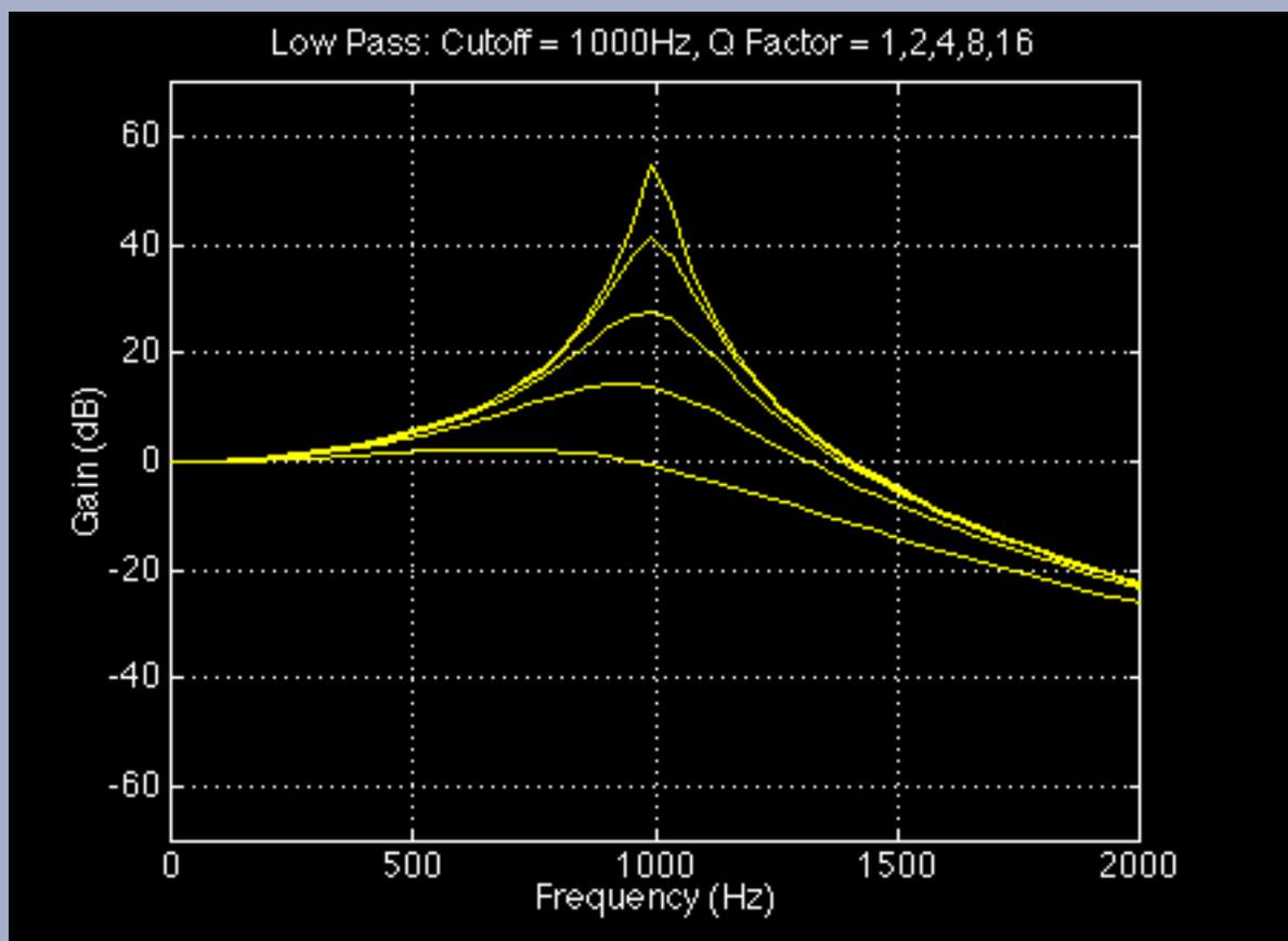
*Low pass filter response curves for different values of Q. A low Q filter has a smooth roll off. A high Q filter has a resonance peak before the cutoff frequency.*
