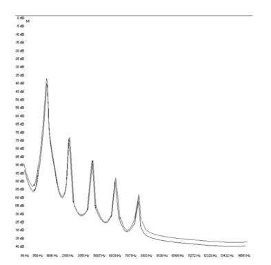
Comparison of Harmonics generated by the filter circuits of the Analog Factory 2.0 and a hardware synthesizer when in self oscillation
