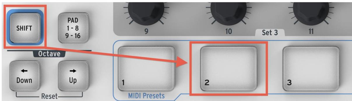
In the picture above the combination of the Shift button and Pad 2 will select Preset #2 from the MiniLab preset memory locations.
