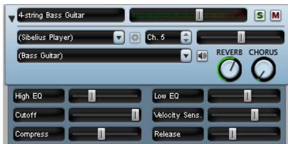
Expand all the staff strips in the Mixer window by **Shift**-clicking on one of the arrowheads to the left of the instrument names.
