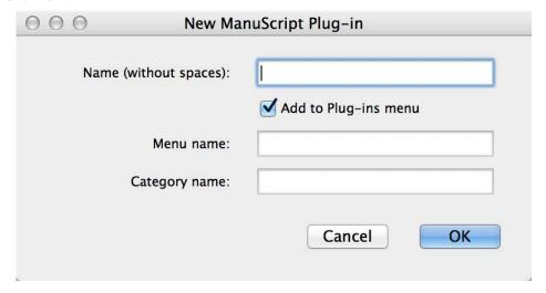
4 You are asked to type the internal name of your plug-in (used as the plug-in's filename), the name that should appear on the menu and the name of the category in which the plug-in should appear, which will determine which ribbon tab it appears on.
