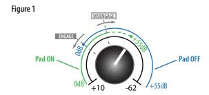
In Auto Pad mode, the two gain ranges in the Aviom preamps overlap. When increasing gain on the console, the Aviom pad is automatically disengaged going from -15 to -16. When decreasing gain, the Aviom pad is engaged going from -7 to -6.
