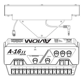
Connect the Cat-5e jumper cable from the MT-X to the A-Net In jack and the TRS jumper cable to the audio output on the Personal Mixer.
