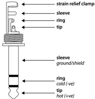
For connection of balanced and unbalanced plugs, ring and sleeve have to be bridged at the stereo plug.
