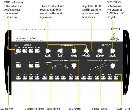
selects the MAIN stereo bus user to listen to selected inputs allows user to mute to selected input channel, stereo linked pair or pre-selected group of channels with meter sets selected input placement within stereo image adjusts level of selected input, stereo pair, group or MAIN stereo bus CHANNEL SELECT buttons each with two LEDs (signal and clip) indicate currently selected single channel, stereo pair or pre-assigned groups
