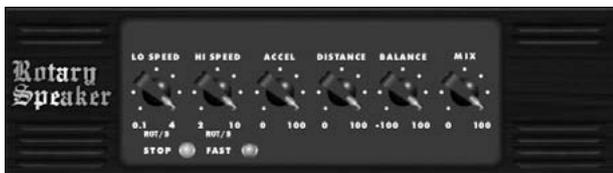
Rotary Speaker emulates the sound of a Leslie rotating speaker. X32's Rotary Speaker provides more flexibility than its electro-mechanical counterpart, and can be used with a variety of instruments, and even vocals, to create a whirling, psychedelic effect.
