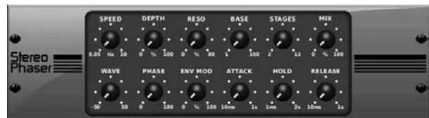
A Stereo Phaser, or phase shifter, applies multiple STAGES of modulated filters to the input signal to create a "notch" in the frequency response, and then applies a MIX with the original for a "swirling" effect. Use X32's Stereo Phaser to add a "spaced-out" sound to vocal or instrument tracks.
