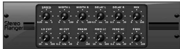
The Flanger emulates the phase-shifting sound (comb-filtering) originally created by applying pressure against the flange of the reel on a tape recorder. This effect creates a unique "wobbly" sound that is quite dramatic when used on vocals and instruments.
