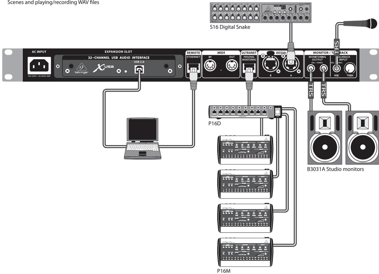
Cabling for all AES50 connections between X32 and S16 stageboxes:
