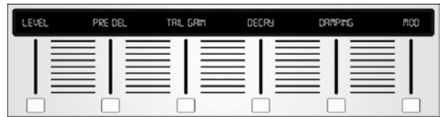
Ambience creates a customizable virtual acoustic space in which to place the elements of a mix. Use Ambience to add warmth and depth without coloring the direct sound. (Inspired by the Lexicon Ambience Algorithm)
