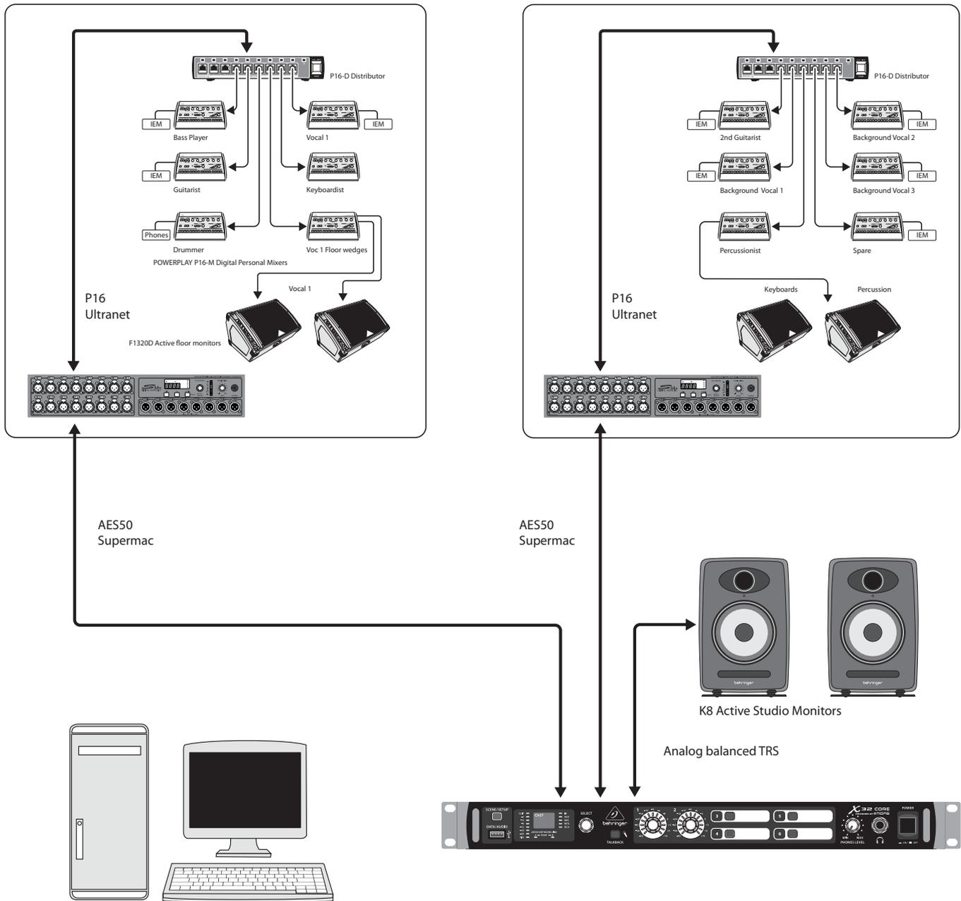
Control room with PC application to run both stage setups from one location through the X32 CORE
