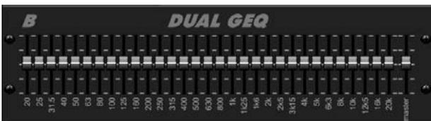
These are standard graphic equalizers that provide 31 bands of adjustment between 20 Hz and 20 kHz. A master volume slider compensates for changes in volume caused by the equalization. A maximum boost or cut of 15 dB is available for each band.
