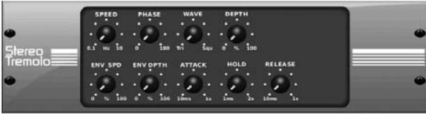
Stereo Tremolo creates an up and down volume change at a constant and even tempo just like the guitar amps of yesteryear. Use X32's Stereo Tremolo to add a unique "surf-music" texture to a vocal or instrument track.
