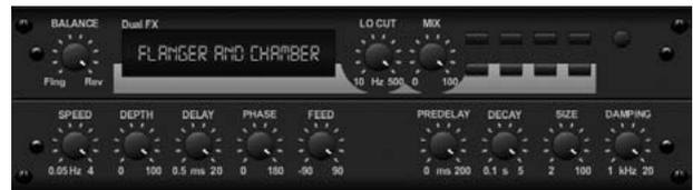
Add the mind-bending, filter-sweeping effect of a state-of-the-art Flanger to the elegant sweetening of a traditional Chamber reverb—all in one FX slot. (Reverb is Inspired by the Lexicon PCM 70)
