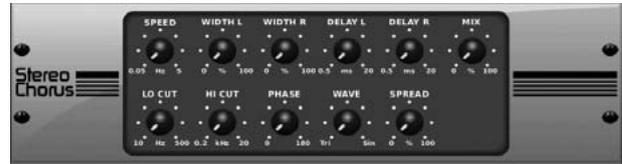
Chorus samples the input, slightly detunes it and mixes it with the original signal to produce a somewhat thicker, shimmering sound. Use it to thicken up background vocals, or to double the sound of brass and woodwind instruments.
