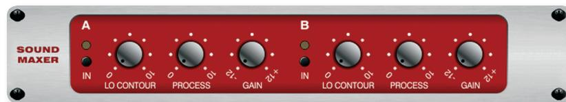
The **SOUND MAXIMIZER** restores natural brilliance and clarity to any audio signal by adjusting the phase and amplitude integrity to reveal more of the natural texture of the sound, which is often hidden when using some effects and equalizers. (Inspired by Sonic Maximizer 482i\*)
