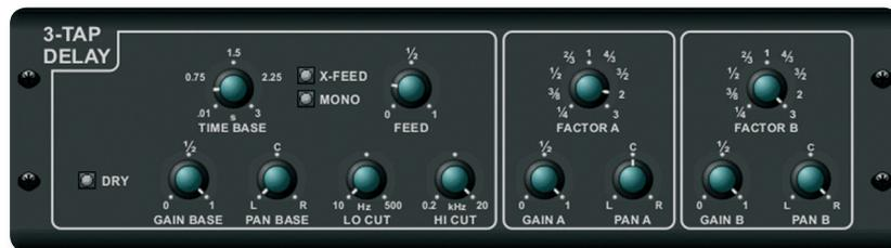
The **3-TAP DELAY** in the X32 PRODUCER records the input signal and then echoes it back after a user-definable period of time and number of repeats. What makes the stereo and triple delay useful and outstanding is the linked tap-timing and musical choice of echo patterns.
