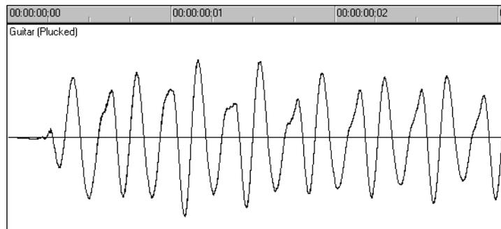
The waveform crosses the zero line twice during each complete vibration. These **zero-crossings** are important in digital audio processing; they are good places to cut waveforms apart and splice them together. If waveforms are cut or spliced at other locations, clicks and pops can occur. The maximum amplitude of the waveform in each vibration is also important: it determines the strength of the vibration, and thus the loudness of the sound.
