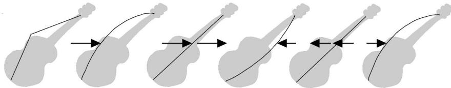
The actual distance the string moves is called its **displacement**. This is proportional to how hard the string is plucked. A greater displacement results in a louder sound.
