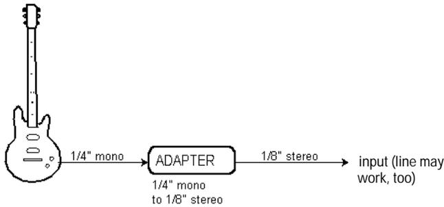
The 1/8" jack should be plugged into the sound card's mic input, although plugging into the line input may also work.
