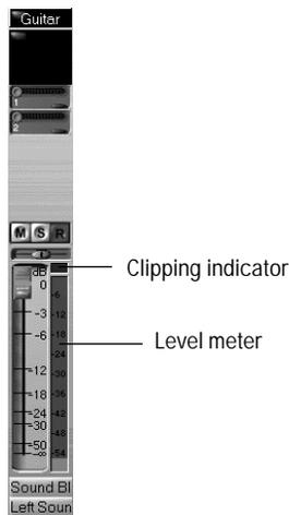
When the audio level exceeds 0dB, some of the audio information is lost. This is known as **overload**. Many sound cards use clipping to deal with an overloaded signal, but clipping can distort the audio signal. As a result, you should avoid letting the meter level exceed 0dB.
