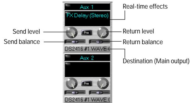
At each main output, all audio data from audio tracks and aux busses that were routed to the main are mixed together and processed by the main's real-time effects. Finally, the data passes through the master volume faders and is sent to the output port, as shown in the following picture:
