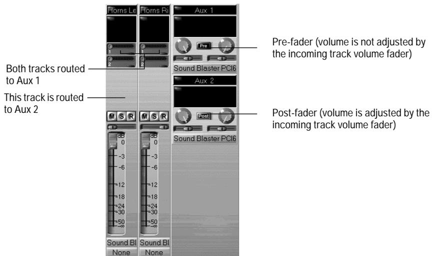
The audio in each aux bus passes through the send level and pan controls, is processed by any real-time effects you have patched, sent through the return level and pan controls, and then sent to the designated main output, in stereo. This is shown in the picture below:
