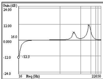
The horizontal axis shows increasing frequency; the vertical axis shows the gain or attenuation at each frequency. If the curve is above the horizontal center line, parts of the signal at that frequency will be boosted; if the curve is below the center line, the signal will be attenuated.
