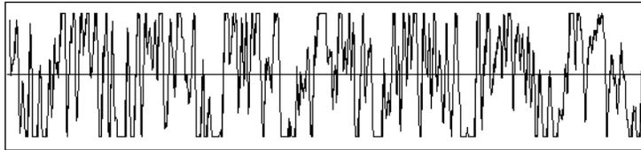
Clipping is not usually desirable and may have unpleasant audible effects. Sudden irregularities in the waveform of any type can cause clicks, pops, and distortion of the original sound.
