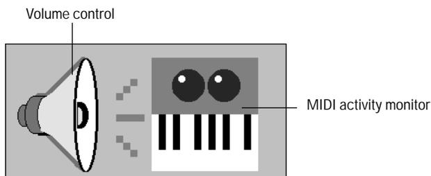
The MIDI activity monitor contains two lights that indicate MIDI input and output. When you play your MIDI keyboard, the first light flashes when each note is pressed, and it flashes again when each note is released. When you play back a project that contains MIDI, the second indicator lights up.
