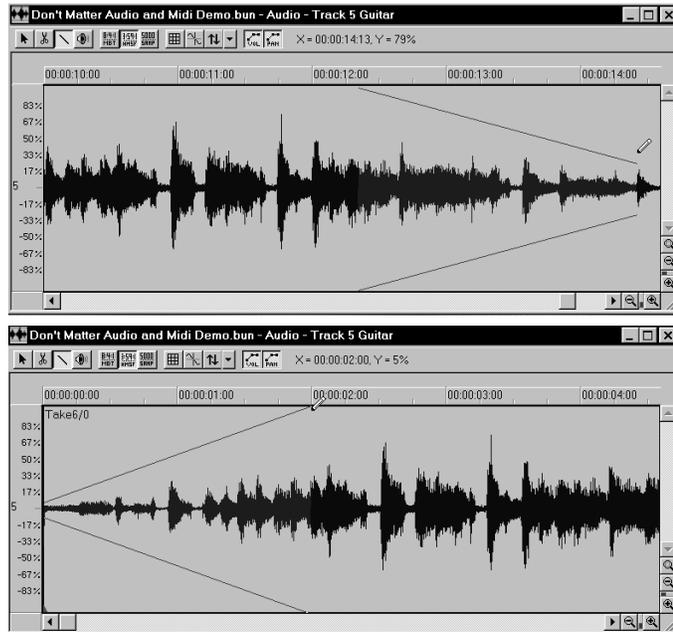
The height of the envelope at each point determines the multiplicative factor that will be applied to the waveform at that point. The zero-crossing line of the waveform corresponds to an envelope height of 0 percent, the maximum amplitude line corresponds to 100 percent. In the first picture, for example, the envelope starts at 100 percent at the left, and fades to 0 percent (silence) at the right. In the second picture, the envelope starts at 0 percent, and swells to 100 percent.
