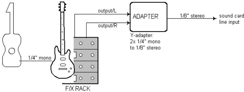
This diagram assumes that the output of the rack is at line level. If it is at pro level instead (+4 dB), and your card does not accept a +4 db input, you will need to attenuate (lower) the F/X rack's signal. To do this, use a mixer between the rack's output and the Y-adapter. If the rack has only a mono output, a 1/4" mono to 1/8" stereo adapter should be used instead of a Y-adapter.
