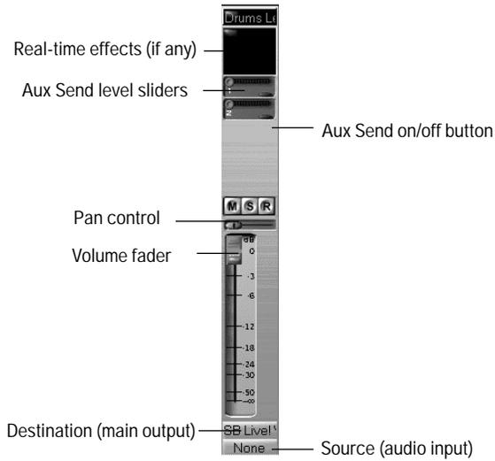
Any audio track can be tapped, before or after the track volume control, and sent to one or more aux busses. An aux bus can tap any number of audio tracks. Each track's data passes through the track's send level knob on its way to the aux bus. This is shown in the diagram below:
