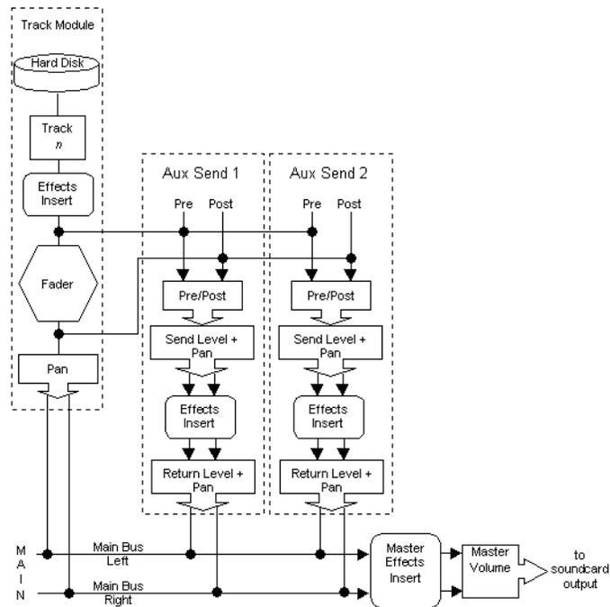
Audio events in each track are processed by any real-time audio effects you have patched in place, passed through the track pan control and volume fader, and then sent to the designated main output, in stereo.
