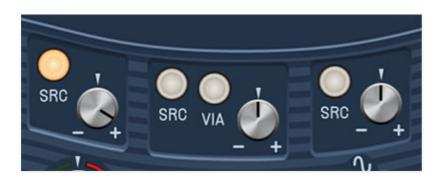
Parameter modulation controls are above or adjacent to many of the oscillator controls. These allow modulation of a control from numerous mod sources. The mod controls are as follows:
