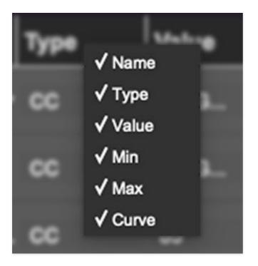
Right-clicking anywhere in the top row (*Name, Type, Value*, etc.) displays the column configuration menu. Checking/unchecking these allows hiding and display of each column. This has no effect on assignments.
