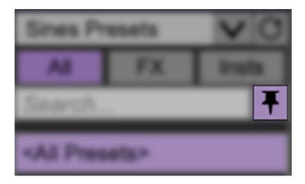
**Pin**- Clicking the push-pin icon locks the patch selection list open, allowing fast and easy browsing and auditioning of patches. Click the icon again to disable pin mode. when in pin mode, the up and down arrow keys can be used to select patches.
