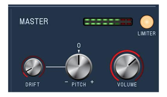
The Master section controls affect the entire instrument globally. **All Master settings are saved with individual patches**.
