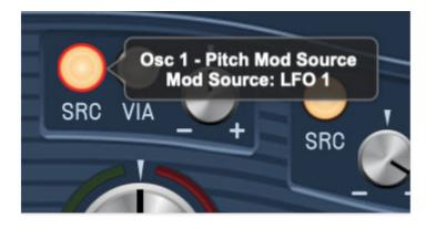
The current mod source is visible in the popup tooltip flag when the mouse is hovered over the *Src* button (You can set how quickly the tooltips display after mouse hover by clicking *Settings gear icon>Interface>Tooltip Delay* in the top purple tool bar). Note that modulation only occurs withing the existing control range; that is, a given control cannot be modulated past its minimum or maximum knob/slider setting.
