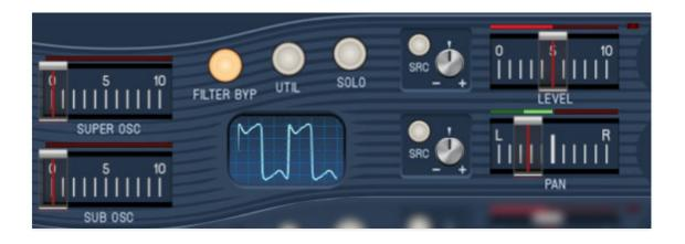
**Super / Sub Oscillator**- The Super Osc and Sub Osc sliders add a sine wave one octave above and one octave below, respectively. **The Super and Sub Oscillators are** *not* **affected by the preceding waveshaping controls**, that is, they remain pure sine waves regardless of the shape of the main oscillator waveform. The *Super* and *Sub* sine waves are really useful for beefing up DX FM-style phase-modulation patches.
