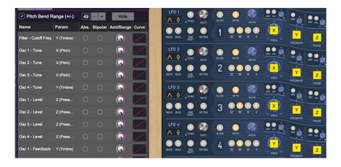
Sines supports MPE, short for "MIDI Polyphonic Expression." It's a specialized MIDI protocol enabling multidimensional controllers for controlling multiple parameters of individual notes. MPE specifies the MIDI messages used for three dimensions of control, regardless of how a particular controller physically expresses them. MIDI channel 1 is used as a master channel for global pitch bend, aftertouch, etc.; MPE utilizes MIDI channels 2-15 for the remaining controller data.
