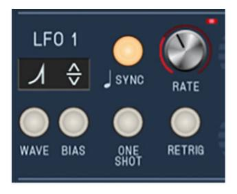
LFO is short for "low-frequency oscillator." The four onboard LFOs generate sub-audio range signals for modulation purposes. The functionality of all four LFOs is identical.
