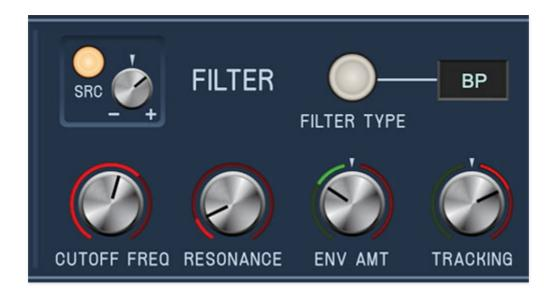
Sines features a resonant multimode filter, including four lowpass modes, highpass, bandpass, and notch modes for all manner of sound sculpting.
