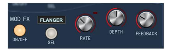
Mod FX features chorus, flanger, and rotary speaker modes. Mod Effects operate in stereo, that is, incoming mono audio will be stereoized, but dry panned audio will maintain its pan position.
