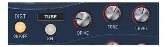
Sines distortion effect operates in dual-mono mode; that is, it doesn't stereoize incoming mono signals, but incoming stereo imaging is maintained - the stereo image isn't summed to mono. You can hear this for yourself by setting up a patch with two or more oscillators and moving the *Pan* sliders.
