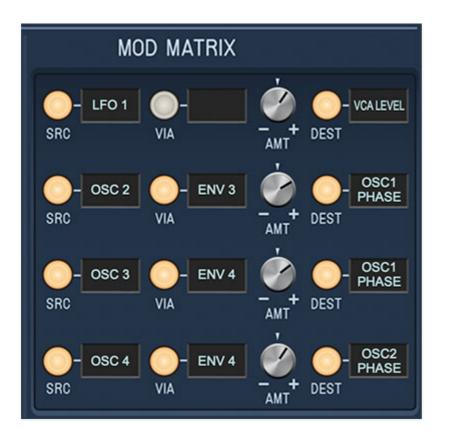
Here's where things get heavy. Sines includes a four-slot mod matrix that allows modulation of almost every single Sines parameter. It works exactly like the individual Parameter Mod boxes explained above, but instead of being tied to the parameter of an adjacent control, each Mod Matrix slot includes a destination parameter.
