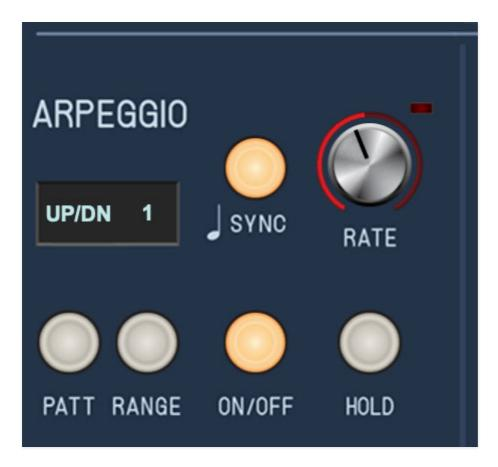
An arpeggiator is basically a step sequencer that plays each note of a chord individually in a pattern across one or more octaves.
