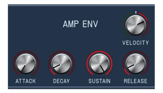
Sines includes four almost-identical envelope generators:dedicated envelopes for the Filter and Amplifier, and two auxiliary envelope generators (Envelope 3 and 4) usable as mod sources for many Sines mod destinations. The dedicated Filter envelope generator is hardwired to the the filter *Cutoff* control, and the Amp Env is hardwired to Sines' onboard VCA for overall amplitude shaping.
