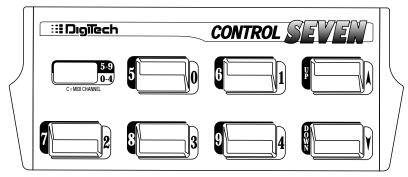
The Program Number/MIDI Channel display is a 4-digit LED display. The pedals perform the program change and bank up/down functions. The back of the unit has a standard 5-pin DIN MIDI jack, and a 3.5mm Power In jack.
