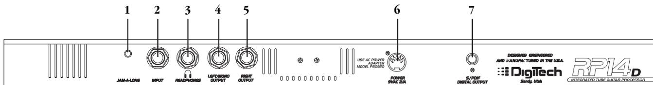
**1. Jam-A-Long Jack** - This is where you connect a tape or CD player in order to jam along with the music, or for the purpose of recording a lick into the Learn-A-Lick phrase recorder. See page 9 for more on using the Jam-A-long and Learn-A-Lick function.
