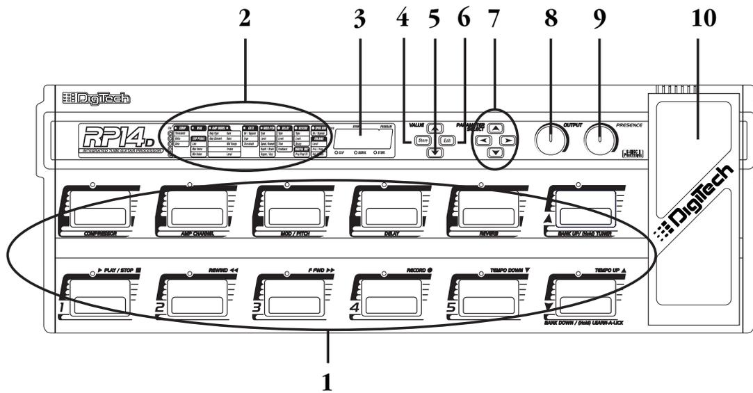
1. **Footswitches** - The footswitches are used to select Programs, change Banks, access the Tuner, turn individual effects on and off, change Amp Channels, select functions in Learn-A-Lick mode, or bypass the RP14D.
