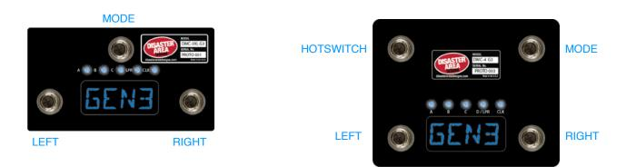
The DMC Gen3 controllers feature a four-character alphanumeric display and five LEDs. The LEDs indicate the bypass status of the connected MIDI devices, the looper record / play state, and the tap or clock pulse.
