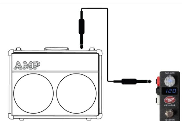
If you're controlling a Strymon pedal, you'll need to set your output's DIP switch to enable the *pull-up* and to connect with a TRS cable.
