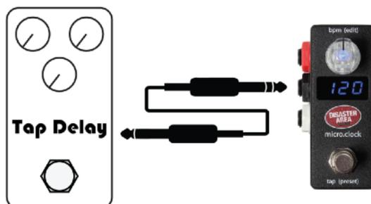
If you are sending taps to a Boss pedal, then you should configure its output to *normally-closed* using the Setup menu.
