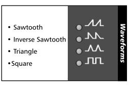
single shot is on, Triangle, Sawtooth, and Inverse Sawtooth all become triggerable envelopes. The Division button allows you to select how many time the waveform envelope will trigger. LFO Speed adjusts the duration of the envelope, and the Filter Momentary triggers the envelope. *Note:* Singleshot does not work when the ENV Follower is selected.
