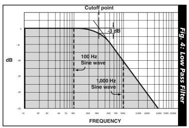
Mono operation by summing the left and right channels before the 4 pole filter. A two pole filter will give you a gentler response, in technical terms it is defined as a 12dB/octave filter. A 4 pole or 24dB/octave filter will give you a much steeper filter response that will sound more pronounced.
