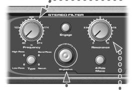
**M**omentary control kicks in the filter unless the Single Shot control is engaged. When Single Shot is on, this button will tyrigger modulation.
