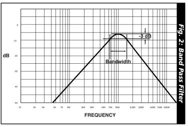
frequency tuning range of the filter covers a 12 octave range from 10 Hz to 40 kHz. The External CV input can control this and has been adjusted to provide standard 1 Volt/Octave response.
