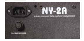
The back panel also contains a fuse holder (2 amp SloBlo) as well as a switch to operate the ground lift. The power connector is a standard 3 pin male plug.
