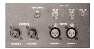
The back panel offers balanced XLR input and output jacks. The input XLR jacks are accompanied by a pair of switches that may be set to allow the selection of a 20 dB pad or to the default 0 dB position.
