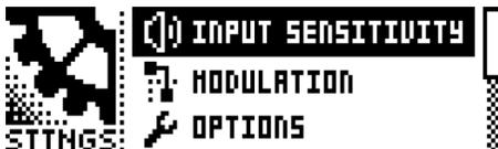
Scroll through the list of settings by using the *PRESET/DATA* knob. Open a highlighted menu by pressing the *PRESET/DATA* knob or [YES]. To change the settings in the menus, first press, and then turn the *PRESET/DATA* knob.
