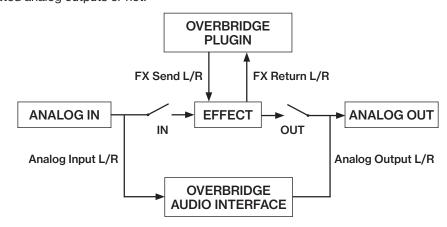
Analog Heat supports 4 channels of audio. Analog Input L/R are routed to the analog in-, and outputs, and can optionally also be routed through the effect. FX Send L/R are always routed to the effect.
