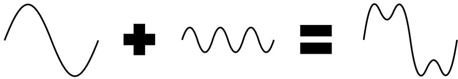
Any waveform can be analyzed as a mixture of sine waves.
