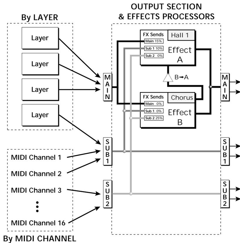
Individual presets or MIDI channels can be routed to the three busses. Note that the signal lines represent stereo signals.
