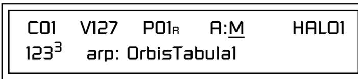
3. Press the **Arp/Beats** button in the Edit section of the front panel to access the master Arpeggiator menu, then use the **data entry control** to scroll to the screen shown below.
