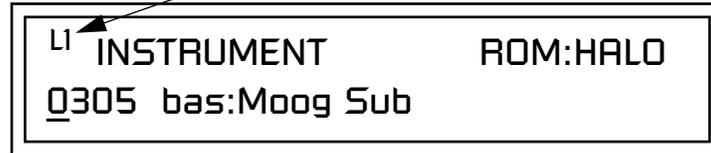
When "All Layers" (A) is selected, the existing parameter value for any field will be displayed if all layers are equal. If the layer parameter values are NOT equal, the value of Layer 1 will be displayed with flashing characters. If you move the data entry control all values will be equal to this new value and the parameter value will no longer flash.
