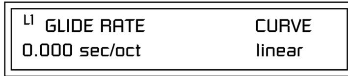
The front panel **Glide Button** LED comes on when the any layer of the current preset has a glide rate greater than 0.000 seconds (regardless of if a PatchCord is connected or not). Pressing the button turns the LED and glide off. Pressing the front panel glide button when all layers are set to a glide of 0.000 turns glide on with a rate of 0.142 seconds/octave.
