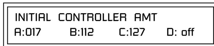
The Initial controller amounts can be set from 000-127 or they can be turned Off. If set to Off, the current controller value is used when the preset is first selected. Setting the Initial Amount to "off" uses the values from the previously selected preset.
