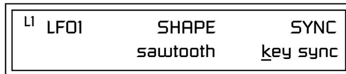
If you modulate the pitch of an instrument, it's easy to visualize the shape of the waveform. For example, the sine wave has a smooth, rolling shape that changes the pitch smoothly. The square waveform changes between two pitches abruptly. A sawtooth waveform increases the pitch smoothly, then abruptly changes back down. The available waveforms are shown below.
