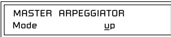
7. Use the **cursor keys** to move the cursor to the *Mode* field (up, down, up/down, forw asgn, backw asgn, forw/backw, random, pattern). Try out the different modes as you play the keyboard.
