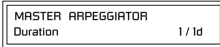
Duration can be used to modify the patterns and increase the possible pattern combinations and variations. Because this parameter limits the length of arpeggiator play time, it can change the arpeggio pattern when the Duration is less than the length of the arpeggio. You can set the arpeggio to repeat continuously using the *Recycle* function described below.
