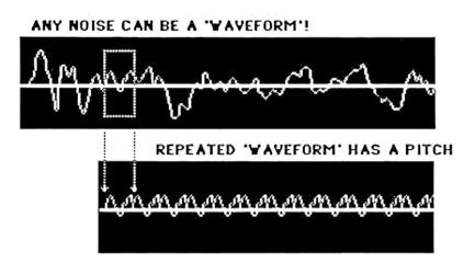
Usually we would like a short loop to have a great resemblance to the original sound! To do that we have to line up the length of the waveform with the length of the loop. Most short loops are exactly one page long, therefore our task is to sample the
