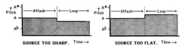
Keep re-sampling and re-tuning until the pitch of the first part of the sound (the part before the loop) matches up exactly with the pitch during the loop. It should become a smooth transition, with no tonal change at the "splice".
