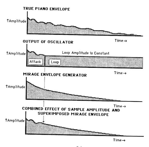
A compressor or a peak limiter will automatically compensate for changing levels in a signal. You can use one to effectively eliminate any envelope from the sound you are sampling making it easier to loop (rapid fluctuations in amplitude are almost as noticable as pitch fluctuations). The envelope generator can then be used to recreate the shape of the sound. This is not always realistic, since the envelope generator may not reproduce all the subtle fluctuations that the compressor took out.
