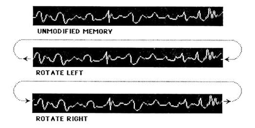
Why would you want to rotate? Loops are very sensitive to the particular sample values at the splice point. Since a loop must always <u>begin</u> on a page boundary, there are usually only a few appropriate places for the loop start point. If the sample at the loop start point doesn't splice cleanly, the particular sample at the start of the page may be changed by rotating, yielding more possibilities for successful loop splices.
