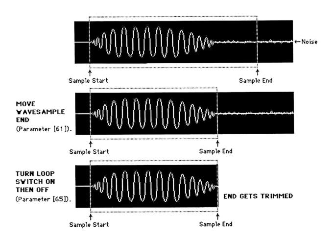
Finally, evaluate the new end point by playing the sound. If there's still some noise, try taking more off. you can do this by going back to the second step. If you cut off too much, the sound will end abruptly (perhaps with a click) and you must reload the untrimmed sound from disk. The trimmed version <u>cannot</u> be restored to its old length. Keep trying different lengths.
