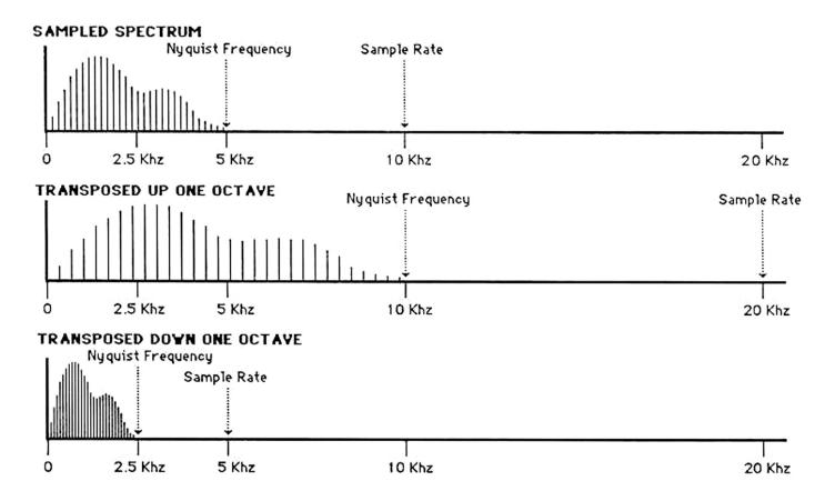
So there is a very simple tradeoff involved in choosing sample rates: sample duration versus frequency response. Sounds with short loops, however, have special requirements for very specific sample rates, as we shall see.
