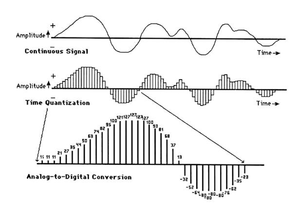
Each of these time steps is represented by a number. The number is the amplitude of the waveform at that instant. This is accomplished with what is, for us, a black box, called an *analog-to-digital converter* (A/D). The analog signal goes in one end, and numbers come out the other. We can control how fast these numbers come out of the A/D--this is called the *sample rate*. For each step, the A/D produces a number by measuring the current amplitude of the signal; it "samples" it.
