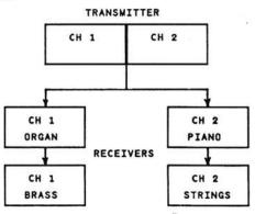
In this configuration, when the lower half of the keyboard is played, we'll get organ and brass. The top half will produce piano and strings. Since we have 16 channels to send and receive, we can also reconfigure the system to look like this:
