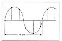
Figure 2. A sine wave measured or sampled 6.25 times per cycle.
