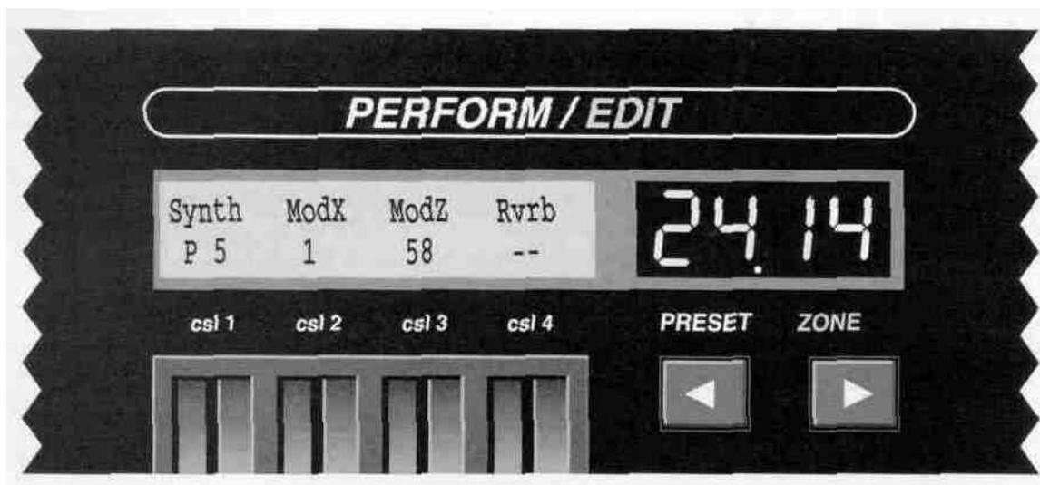
The PROGRAM screen (and also VOLUME and TRANSPOSE screens) display settings for four zones at once. Note that there are now two zone digits (14) indicating that you are viewing zones 1 through 4.
