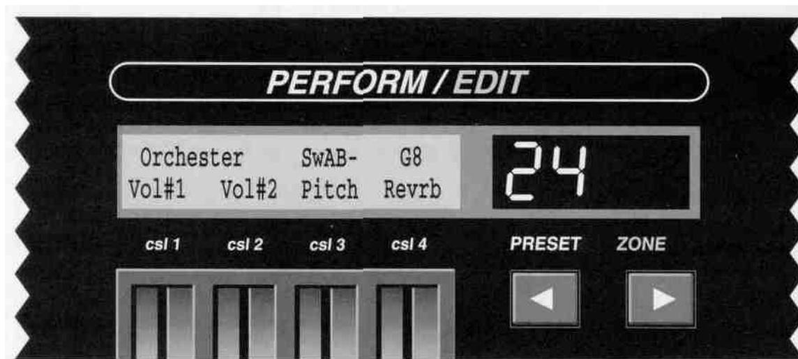
parameters shown. The current value of each parameter appears below the parameter name, and may be changed with the corresponding control slider (while in Edit Mode, any MIDI control functions assigned to a control slider are disabled). The zone digit is present because these functions are zone-programmable (when editing a zone-programmable function, be sure that the correct number is displayed or the wrong zone may be inadvertently changed).
