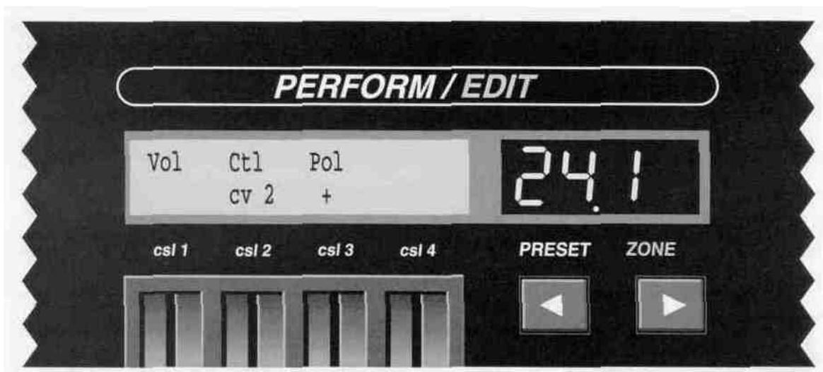
Control slider 2 is used to select the source of volume control. Select from any of the four control sliders (in Perform Mode), control voltage input 1 or 2, Wheel A or B. If no adjustments are required during performance, select None.
