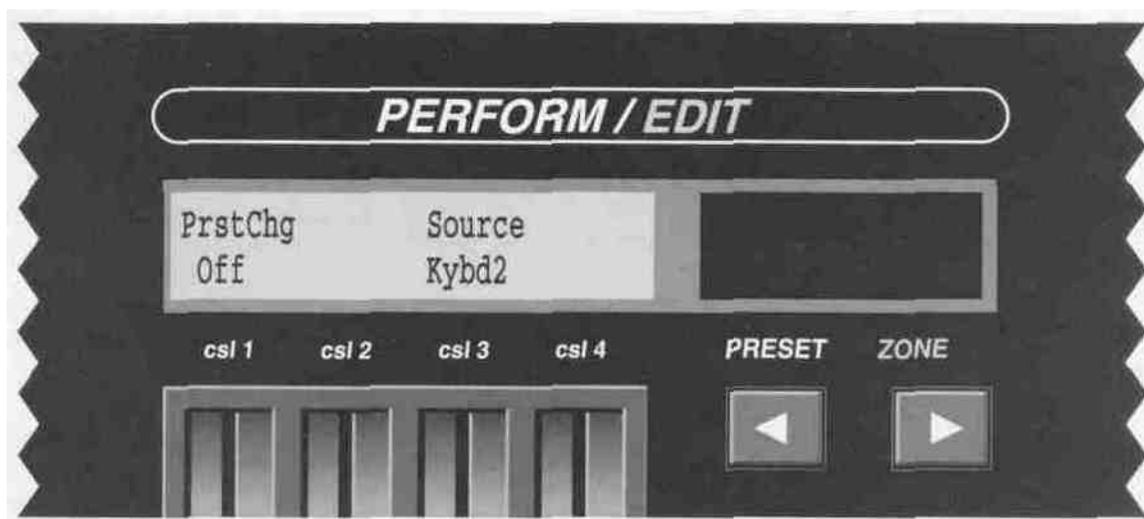
Control Slider 1 is used to enable SL-2001 preset changes via MIDI program change commands. Slider 3 is used to select the device from which the SL-2001 will accept program change commands. Program changes from all input devices will be accepted by selecting All on Slider 3.
