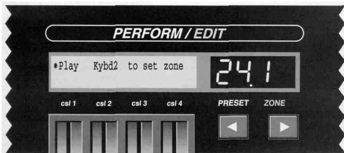
Press the two keys that correspond to the highest and lowest notes desired for the zone. You must play these notes on the instrument specified on the screen. After the second note is pressed, the display will automatically revert to the main ZONE screen with the new settings as programmed.
