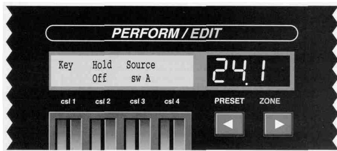
Control Slider 2 turns on the Key Hold function. Select a control source using Slider 3. The control source will usually be assigned to one of the local switches A, B, or C, and activated with the footswitch.
