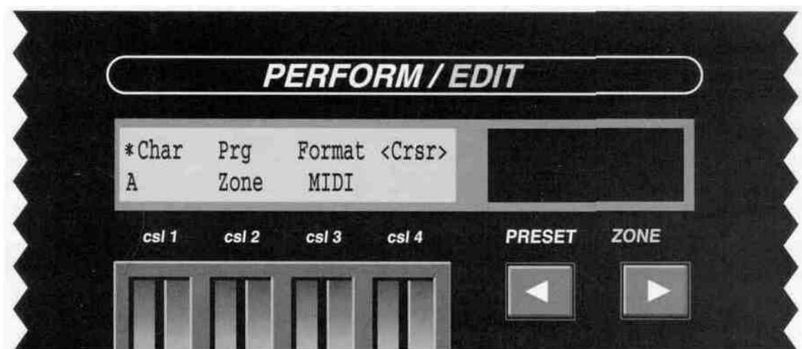
As before, the 5-character device name is entered using Control Slider 1 to select the character and the arrow switches to move the cursor position (characters may also be selected by pressing the appropriate keys on the SL-2001 keyboard). Because we are installing an output device (MIDI OUT A was selected as the port) there are two additional parameters that must be set.
