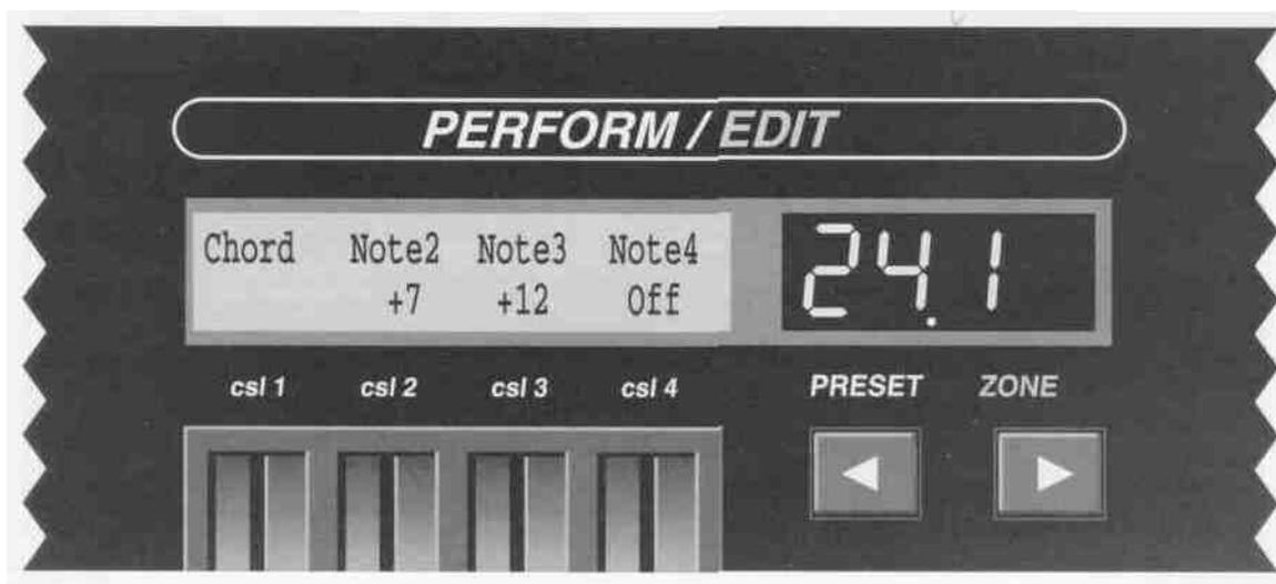
If Control Slider 2 is changed from the Off position, a second note message will be created for every note message received by the zone. A third and fourth note may be introduced using Control Sliders 3 and 4. The control slider settings determine the transpose interval for each of the additional notes. This interval is added to the overall transposition value set in the TRANSPOSE screen. Any notes that are transposed out of the normal MIDI note range will not sound.
