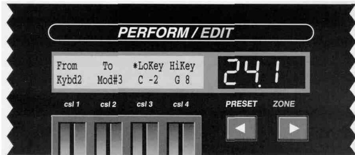
The example screen above shows Zone 1 configured to pass MIDI information from a keyboard (Kybd2) to a sound module (Mod#3). To change the zone's input assignment, move Control Slider 1 until the desired device name appears. To change the zone destination, move control slider number 2.
