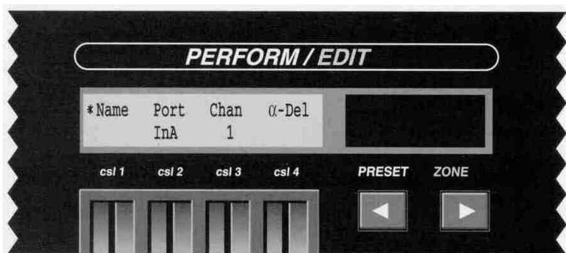
1. Using Control Slider 2, set the Port parameter to IN A. This means that the keyboard we are installing is physically connected to MIDI IN A of the SL-2001.
