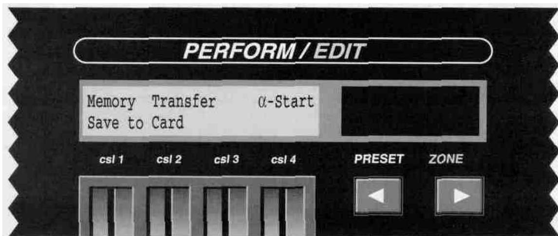
Use Control Slider 1 to select either a *Save* or *Load* operation. If presets are to be saved to the card, the Write Protect switch on the card must be set to Enable. The Alpha switch is used to start execution of the operation. When finished with the card save operation, set the switch back to Protect.
