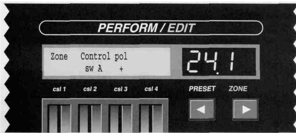
While creating or editing a preset, it is often desirable to turn off some of the zones so that the effects of the edit are more clearly audible. The zones may also be controlled by the five local switches (A, B, C, Star, and Alpha). The ZONE CTL screen is used to select the source of control for the zone.
