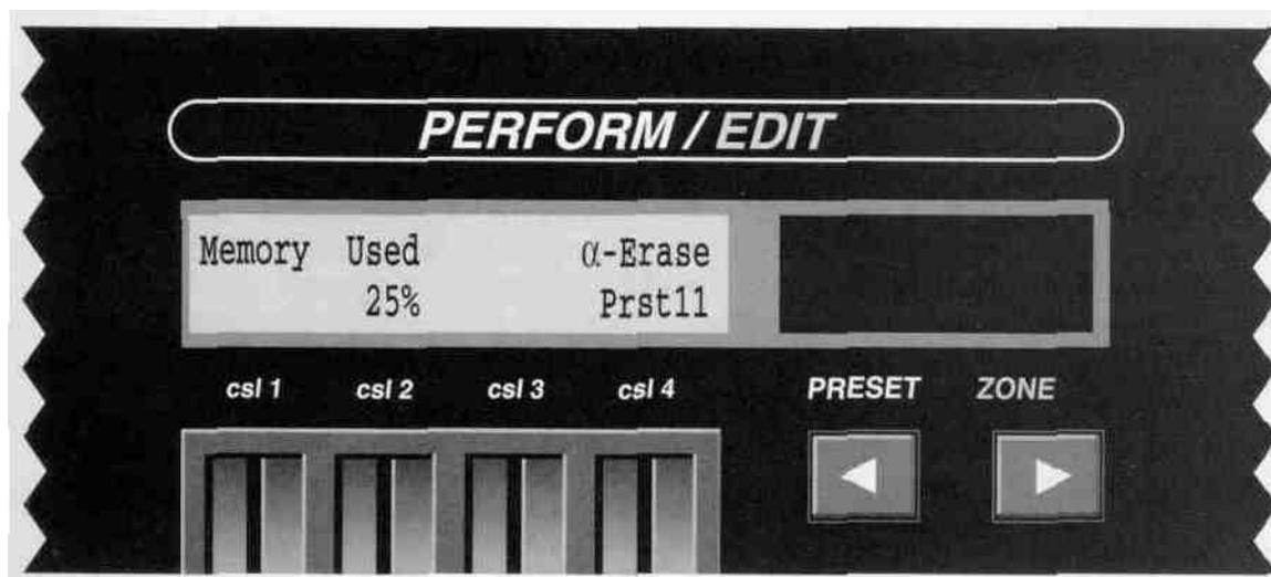
The SL-2001 uses a dynamic memory allocation scheme, which means that the storage space for a preset is dependent on the number of functions that are active in that preset. It is possible (but very unlikely) that the memory space will become full before all presets have been programmed. The Memory Used screen displays the percentage of memory that has been programmed.
