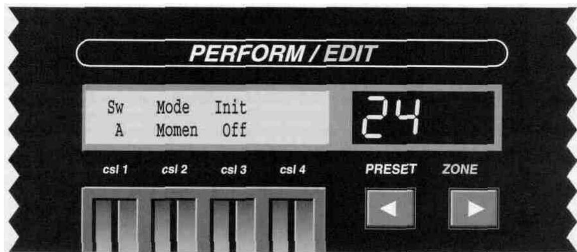
Use Control Slider 1 to select the name of the switch. Control Slider 2 sets the mode (*Toggle or Momentary*). In Toggle Mode, a switch will change state every time the footswitch is pressed and released. In Momentary Mode, the switch will change state when the footswitch is first pressed, and then revert to its original state when the footswitch is released. Control Slider 3 is used to set the initial state of each switch as the preset is entered.
