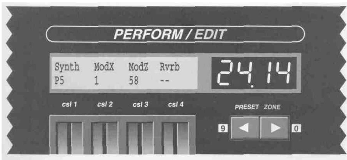
If a zone is bypassed, the top line of this screen will indicate the output port to which the path is assigned. Program change commands cannot be issued from a bypassed zone.
