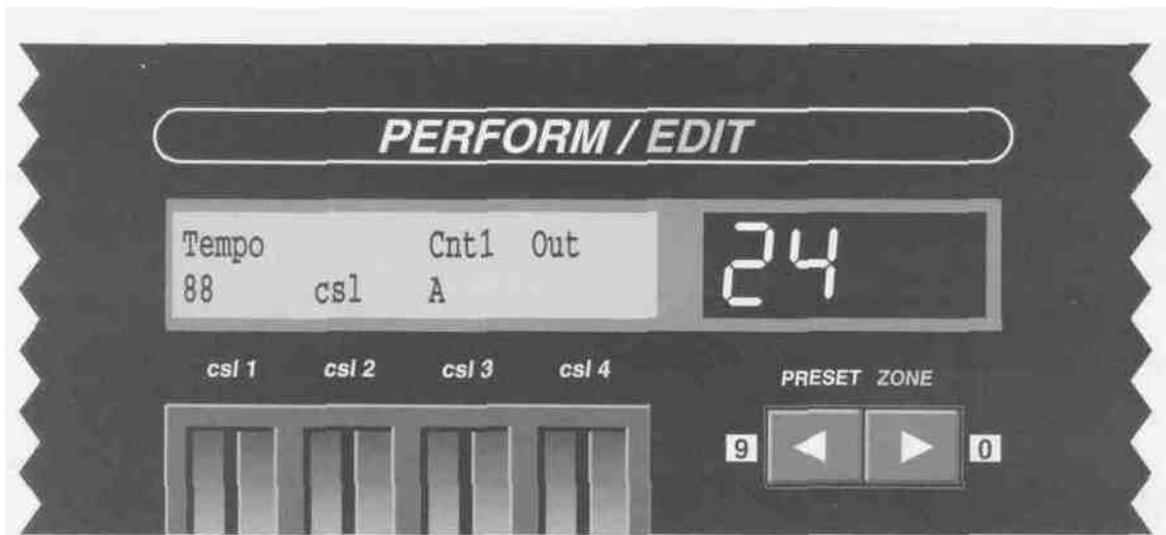
A direct program change feature is available which allows faster access to any program number. PRESET switches 1 through 8 and the left/right arrow switches are used as a keypad to enter the desired number (the left/right arrow switches represent the numerals 9 and 0). To use this feature, first press and hold the ZONE switch (1-8) that you wish to program.
