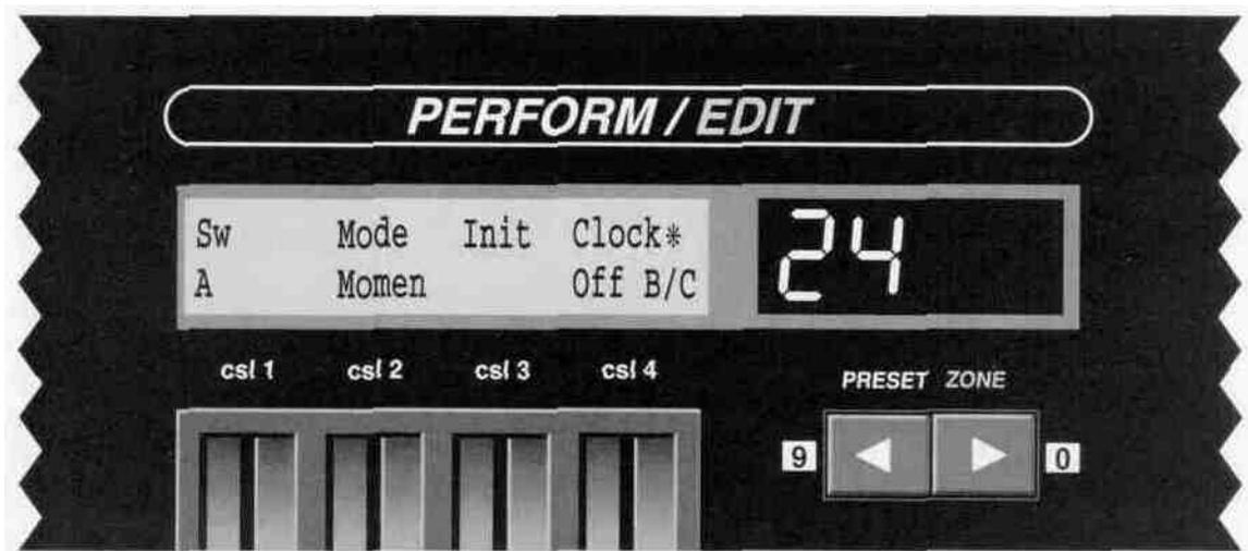
Use Control Slider 1 to select the name of the switch. Control Slider 2 sets the mode (Toggle or Momentary).
