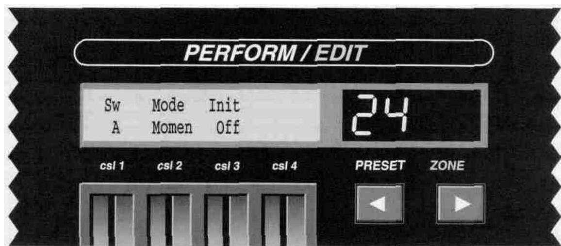
Use Control Slider 1 to select the name of the switch. Control Slider 2 sets the mode (*Toggle or Momentary*). In Toggle Mode, a switch will change state every time the footswitch is pressed and released. In Momentary Mode, the switch will change state when the footswitch is first pressed, and then revert to its original state when the footswitch is released. Control Slider 3 is used to set the initial state of each switch as the preset is entered.
