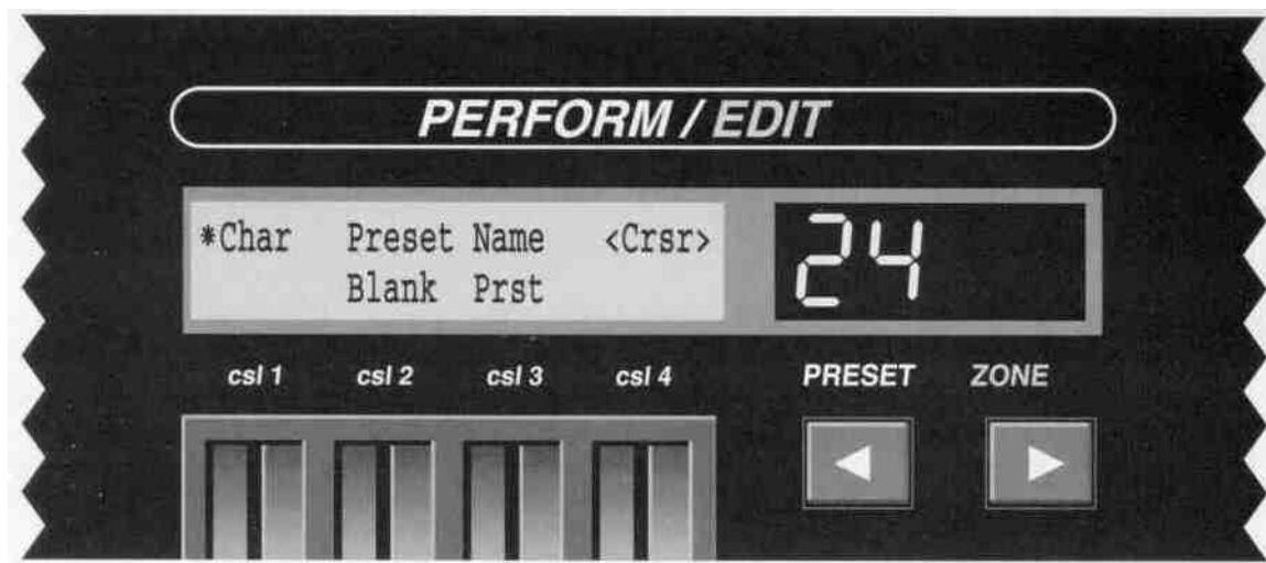
Upon entering this screen, a flashing character will indicate the current position of the cursor. Use Control Slider 1 to select the desired character for this position, or press the appropriate key on the SL-2001 keyboard. To change the position of the cursor, use the left and right arrow switches (< >).
