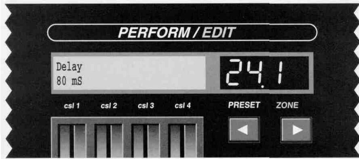
Use Control Slider 1 to select the delay time. This value will be displayed as milliseconds (mS, one thousandth of a second) or as seconds. Maximum delay setting is 10 seconds.
