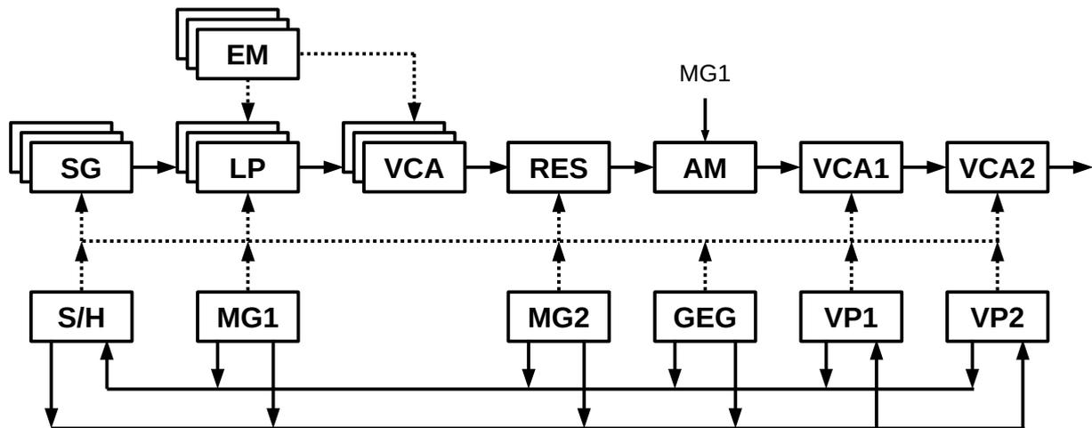
As you can see from the block diagram, there are many signal (solid) and modulation (dashed) paths between the various modules. The configuration is pretty flexible and can be reconfigured in the *Patch Bay*.
