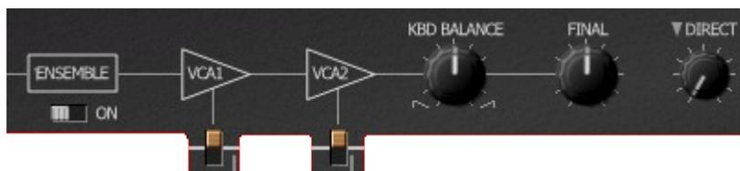
loudness contour by the General Envelope Generator and Voltage Processor 1 (both VCAs have respective switches to enable these modulation sources) but nothing prevents you from patching your own sources via the Patch Bay.
