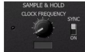
The "SYNC" switch (called "SYNCHRO" on the PS-3100) is bit curious. KORG's original documentation states that "*when the sampled frequency is near the clock frequency multiplied by an integer, the clock is synchronized*". Well, better check it out by yourself. Fact is that a regular/periodic input signal can produce some regular, repetitive output while noise will create random patterns. In any case the SYNC function is disabled when the S/H clock is synchronized to the host tempo.
