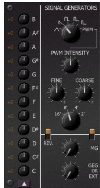
An interesting feature is the *micro-tuning* option. Each of the 12 keys can be tuned individually, allowing for other (not necessarily well-tempered) tunings like *Pythagorean* or *Wendy Carlos' Super Just* tuning etc. The small button at the bottom of the tuning knobs opens a menu with 14 predefined micro-tuning templates. Here it is also possible to load and/or save the tuning settings from/to a Scala (\*.scl) file.
