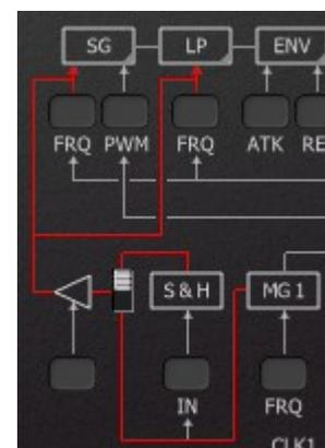
Furthermore, in contrary to the FB-3100 the PS-3100 does not offer an individual outlet of the MG1 signal; the outlet labeled "MG1" on the original PS-3100 panel is in fact equivalent to the "MG" signal on the FB-3100.
