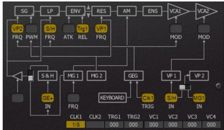
Strictly speaking there are two types of sources and targets: *modulations* and *triggers*. For example the "ATK" target of the EM continuously modulates the Attack time while the "REL" target waits for a trigger signal to release the envelopes.
