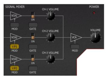
Finally, the total signal is sent again through a final VCA. Note that the final output is a stereo signal since the output of each block can be placed in the stereo panorama. On the PS-3300, you would need a separate stereo mixer for this.
