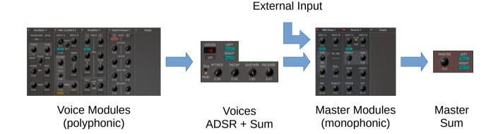
The voice signals generated by the Voice modules are shaped by individual ADSR envelope generators and then summed up to form the *Voices Sum* stereo signal. This signal along with an external input signal can be used to feed the Master modules. The final output can then be selected from the output of a Master module (if applicable) or the *Voices Sum* signal.
