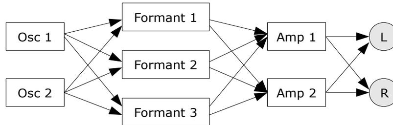
amplifiers with panorama control which are connected to the main stereo output bus.
