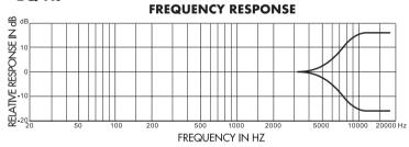
The high EQ control is a shelving EQ. What this means is that it boosts or cuts from 10kHz and everything above that. Turn it up to bring out the breath of a vocal or the high overtones of the cymbals. Turn it down to reduce finger squeaks on a guitar or bass.
