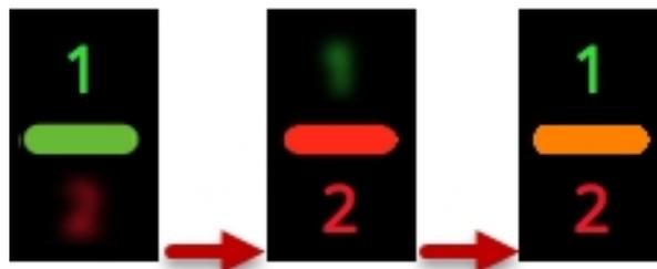
Figure 8: Pressing the touch zone successively will select (in this example) Output 1, Output 2, or Stereo Output 1/2
