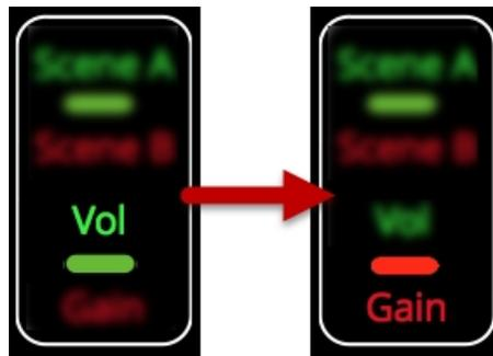
Figure 7: Press once to toggle between Volume display and Gain display modes.
