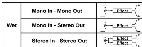
The possible routing of effect signal inputs and outputs is indicated in the upper left corner of the block diagram.
