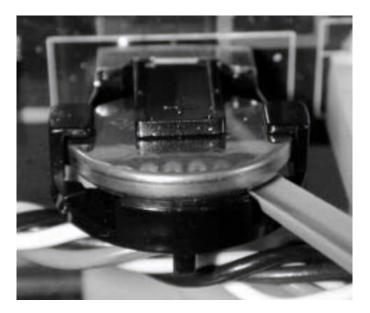
Figure A-1 Freeing battery from retaining clip
