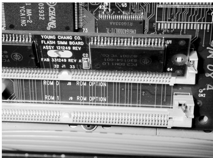
**Figure 9 PCR-1 board properly installed on PCX-1 board**
