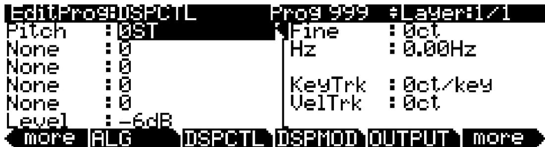
You'll recognize the common DSP control parameters, along with several other parameters. Keep in mind that there's a set of common control parameters for each of the DSP functions; in this case we're describing them only as they apply to the pitch control function.
