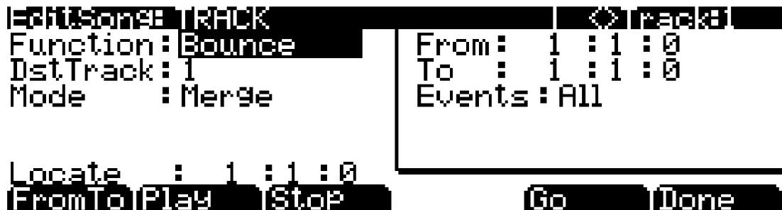
You will notice that the page is divided into two halves, with the right half being a separate box. This is called the Region/ Criteria box. The parameters in this box are used to select the range of events (from a start Bar and Beat to and end Bar and Beat) for modification, as well as which types of events function will affect.
