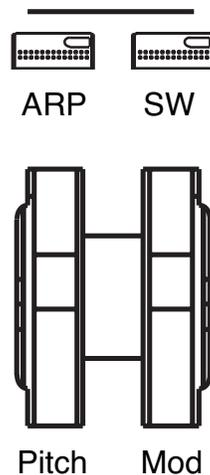
To the left of the PC3's keyboard are the Pitch Wheel and the Mod Wheel, as well as the SW and Arp buttons.
