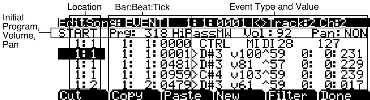
The top line of the page displays the current song position in the center, and the currently selected track and corresponding channel on the right. Use the **Chan/Layer** buttons to select an active track to view and edit the MIDI events recorded on it.
