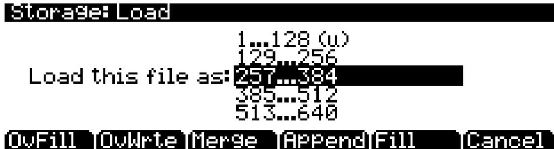
The soft buttons control the mode for loading and renumbering of objects from the file. Here's how they work:
