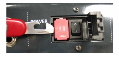
If there is only one fuse in the fuse holder, you must remove the metal clip on the empty side.
