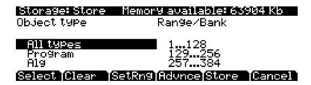
At the top right of the page, the display shows how much memory is available in the current storage device. Along the bottom of the page are the Store page's six soft buttons. Below is a description of the function of each soft button:
