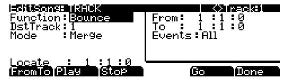
You will notice that the page is divided into two halves, with the right half being a separate box This is called the Region/Criteria box. The parameters in this box are used to select the range of events (from a start Bar and Beat to and end Bar and Beat) for modification, as well as which types of events function will affect.
