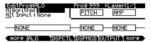
The DSP functions are represented by the rectangular blocks. The lines connecting the blocks together indicates the flow of the digital signal from left to right; they represent what we call the "wire" of the algorithm: the actual physical path that the signal follows through the algorithm. Selecting different algorithms can be compared to connecting different DSP functions with different wiring diagrams.
