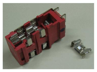
Remove the fuse. Install two 250 mA fast blow fuses for 230V or two 500 mA fast blow fuses for 115V, one on each side of the fuse holder.
