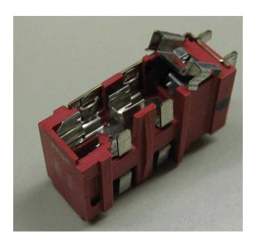
The clip removed from the fuse holder:
