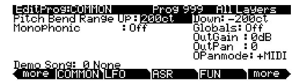
Notice that when the Monophonic parameter is set to its default value of **Off**, the four monophonic parameters do not appear on the page.
