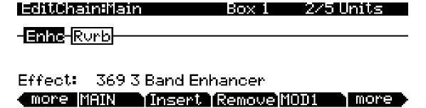
At the top right of the display is the number of DSP units used by the currently selected effect-box, and by the Chain as a whole. **2/5 Units** indicates that the current effect-box is using two DSP units and the Chain is using a total of five DSP units for all of its effects. There are a total of 16 units available for all of the Chains that are currently loaded by programs and any active Aux overrides from Setup/Song/Effects mode.
