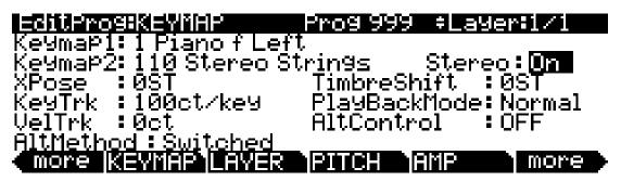
An additional Keymap parameter appears. The two keymap parameters are distinguished as Keymap 1 and Keymap 2. The KEYMAP page parameters will affect both keymaps. When the Stereo parameter is set to **On**, the OUTPUT page for the current layer will show an additional pair of Pan parameters.
