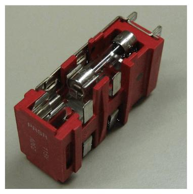
Replace the fuse holder in the power entry module with the indicator for the desired voltage towards the edge of the module, away from the power switch. Close the fuse holder cover, and check that the desired voltage indication shows through the hole. Replace the power cord.
