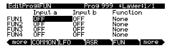
There are three parameters for each FUN. Inputs **a** and **b** can be any control source from the Control Source list. The control sources you want to combine are the ones you'll assign as the values for these parameters.
