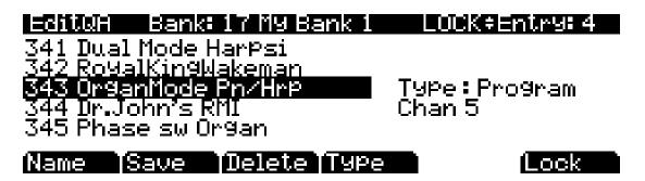
The top line gives you the usual mode reminder, the current QA bank, and the current entry. The cursor highlights the object (program or setup) that's stored in the current entry.
