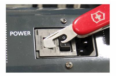
Pull up gently to open the fuse holder cover. The cover is hinged next to the power cord connection.
