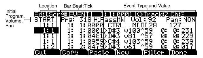
The top line of the page displays the current song position in the center, and the currently selected track and corresponding channel on the right. Use the **Chan/Layer** buttons to select an active track to view and edit the MIDI events recorded on it.
