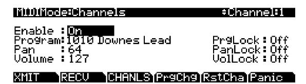
Press the **CHANLS** soft button to select the CHANNELS page, where you can define numerous parameters for each MIDI channel independently. Use the **Chan/Layer** buttons to select the MIDI channel you wish to work on.
