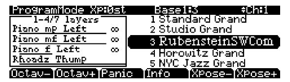
The first time you power up (or after a reset), your instrument will be set to operate on MIDI Channel 1 (as shown at the far right of the top line above).
