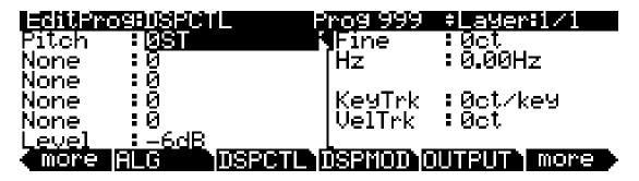
You'll recognize the common DSP control parameters, along with several other parameters. Keep in mind that there's a set of common control parameters for each of the DSP functions; in this case we're describing them only as they apply to the pitch control function.
