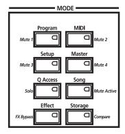
When you press a mode button, its LED lights up to indicate that the mode has been selected. If pressing a mode button does not light its LED, press the **Exit** button one or more times, then try again.
