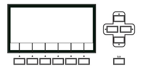
Programming the PC3 involves selecting various parameters and changing their values. Select parameters by highlighting their values with the cursor. You can change the highlighted value with any of the data entry methods described in the data entry section below.
