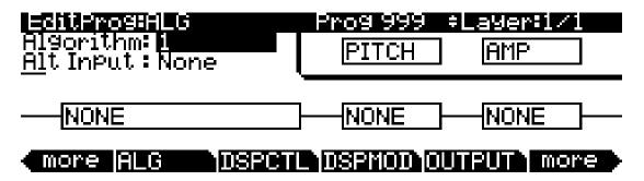
The central portion of the page shows the algorithm for the currently selected layer. You see the number of the algorithm (from 1 to 28, 101 to 131, and the IDs for any user-defined algorithms) and a graphic representation of the signal path, as well as the currently selected DSP functions within the signal path.
