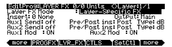
All of the Layer-Specific FX mode parameters have the same functions and ranges of values as their corresponding parameters on the PROGFX page. See *The Program FX (PROGFX)*Page on page 6-46 for more information on these parameters.
