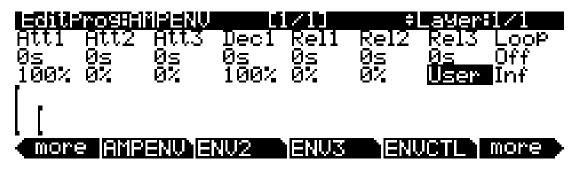
You'll tweak the parameters on the AMPENV page when you want to shape the amplitude characteristics of your sounds. A graphic view of the amplitude envelope will appear on the display to give you a visual sense of the envelope's characteristics. The dots along the envelope graphic indicate the breakpoints between the envelope's various segments. The small horizontal arrow represents the end of the decay section. The small downward-pointing arrow represents the beginning of the release section.
