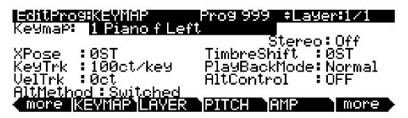
The top line of the display gives you the usual reminder of your location. It also tells you which layer you're viewing, and how many layers there are in the program. You can use the **Chan/Layer** buttons to scroll through the layers, if the program has more than one.
