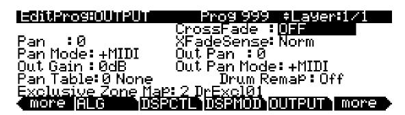
These parameters are analogous to the output parameters on the COMMON page, but are layer-specific—the COMMON output parameters apply to all layers. You can use the output parameters on the OUTPUT page to adjust the panning and gain of the *post-FX signal of the current layer*.
