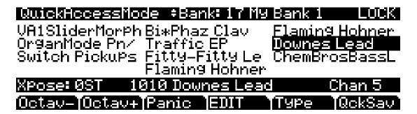
The top line of the page—from left to right—displays you the current mode, the current QA bank, and the Locked status of the current QA bank. The word "LOCK" displayed in the upper right-hand corner of the screen indicates that the current QA bank is locked—more on locked QA banks in *Locking the Current QA Bank*.
