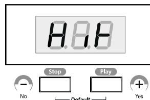
< Figure 4-17 Setting the Highest Note for the Zone >
