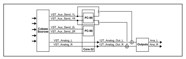
Note also that, as 12T\_Analog\_Out\_L and 12T\_Analog\_Out\_R are selected as PC-90s destinations, the audio is summed with the outputs of Cubase VST, which are also routed to the analog outputs. This allows monitoring of PC-90 reverb and all audio from VST through the same outputs of the interface.
