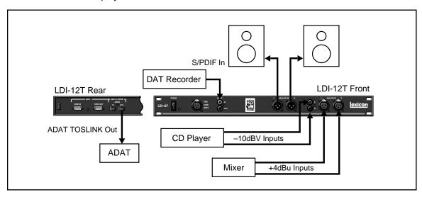
S/PDIF connections can be made to any digital device such as the send/returns of a digital signal processor.
