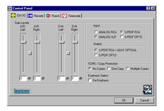
**Gain Levels** are controlled by the on screen faders with the gain displayed numerically at the bottom. A gain of 0dB sets unity gain from XLR input to XLR output, where +4dBu is 14dB below digital full-scale. (For the RCA inputs, 0dB corresponds to -10dBV, 14dB below digital full-scale.)
