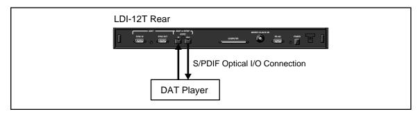
The LDI-12T can accept different input and output formats as shown below. This configuration can be used for format conversion from optical S/PDIF to coaxial (RCA) S/PDIF and to provide flexible routing.
