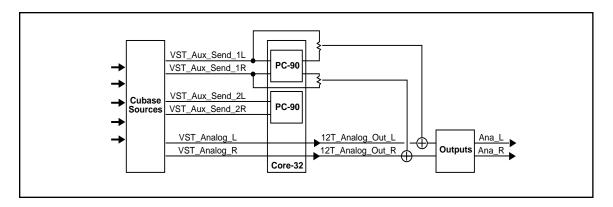
As 12T\_Analog\_Out\_L and 12T\_Analog\_Out\_R are selected as destinations, PC-90 audio is summed with the outputs of Cubase VST, which are also routed to the analog outputs. This allows monitoring of PC-90 reverb and all audio from VST through the same outputs of the interface.
