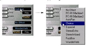
Selecting a PC-90 machine in this pulldownwill activate a PC-90 Rack Xpander within VST.
