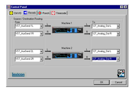
The reverb page allows you to route the PC-90's two DSP engines independently through any of the connectors of your audio interface.
