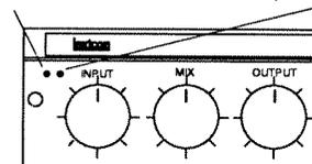
**Note:** If the PEAK LED flashes with no input present (i.e., during reverb decay or delay line feedback, it indicates processor overload is occurring.
