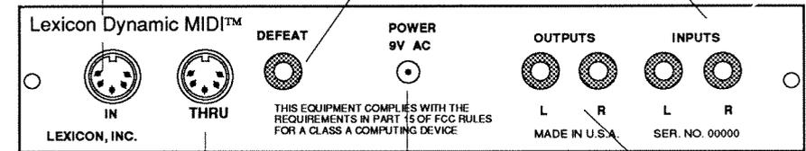
**MIDI THRU.** Any data received at the MIDI IN connector is sent here without change. An internal jumper can be set to change this into a MIDI OUT connector.
