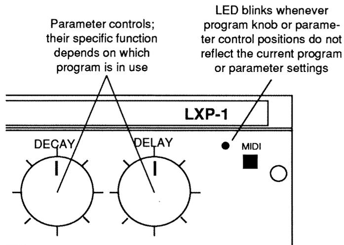
When you load a new program, the front-panel MIDI indicator blinks to let you know that the position of one or both of the parameter controls does not reflect its actual setting. As soon as you move a knob, the parameter snaps to the new setting you've selected. Once you've moved both parameter knobs, the knob positions accurately reflect the current setting, so the MIDI indicator stops blinking.
