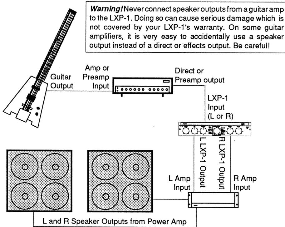
**Connection between instrument preamp and power amplifier(s)**
