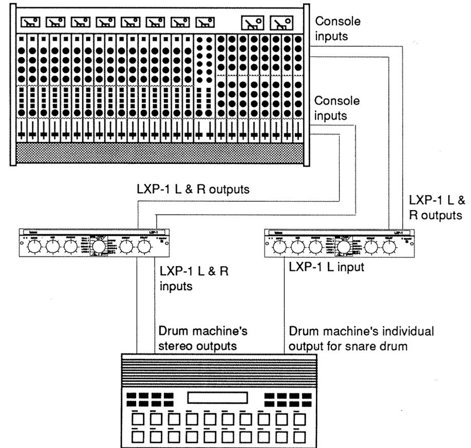
**Connection between drum machine and console**
