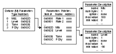
For example, in the "Detune (M)" effect, "Tune" is the third parameter. After a pointer is initialized to the beginning of the pitch "32 byte parameter data" array, it must be incremented past the first and second parameters' data to get to the "Tune" data.
