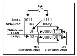
As in all other cases in the MPX 1, the less-significant portion of the byte is transmitted first. 16-bit "words" (2 bytes) are sent low nibble of the low byte, followed by high nibble of the low byte, low nibble of the high byte, then high nibble of the high byte.
