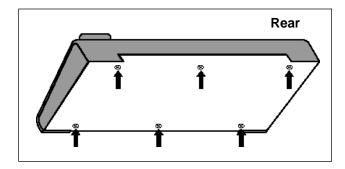
Remove the bottom plate and put it aside.
