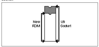
Avoid bending any pins. When the ROM is inserted, carefully inspect each pin to be sure that it has not been bent.
