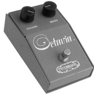
The Octavia uses an audio output transformer and two germanium diodes to rectify (a fancy word for whack) the bass signal, thus creating the high octave type sound. For our model, we studied the sweet-sounding original pictured here. We knew we had a keeper when every guitarist and bassist in the building wanted to take it home for a little of their own after hours “research.”
