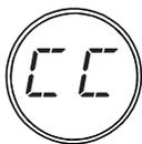
Another feature of using MIDI with your Filter Pro is the ability to control virtually every parameter of each effect in real-time using MIDI Continuous Controllers (henceforth referred to as MIDI CC#). There are actually 127 of these little devils to go around, which is more than enough to control everything your Filter Pro can do (and then some!).
