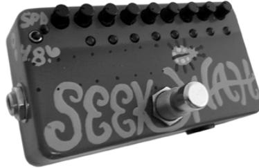
The Seek Wah is a box that contains 8 “parked wah” filters that can be set at varying positions and then sequenced through, creating a pulsating hypnotic vibe (with no detectable side effects!). In our ode to this unique creation, we give you the Seeker. Here’s how it works:
