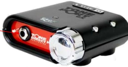
**Guitar/Bass** - To input your electric guitar or bass, plug it in here using a standard 1/4-inch TS instrument cable.
