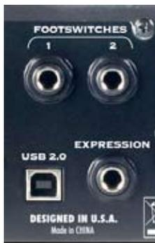
You can use up to 2 on/off toggle or momentary footswitches, and 1 expression pedal to remotely control functions in the GearBox software, such as stomp effects or wah level. You can also configure footswitches and the expression pedal to send MIDI commands, which can be useful for controlling your recording software's transport.
