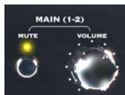
Main Outputs 1-2 are controlled by a main volume knob and main mute button. The volume knob is an analog level control and does not affect any level being sent to your computer. When Mute is engaged, as solid amber LED illuminates, blinking about once every 2 seconds.
