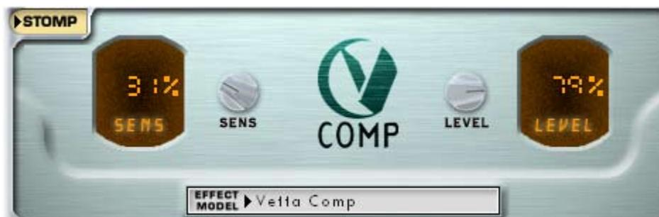
The GearBox Stomp effect also includes the Vetta Comp compressor that runs “pre” (before) the amp processing, which can give a different kind of sound than the dedicated Comp effect which always runs “post” (after) the amp processing.
