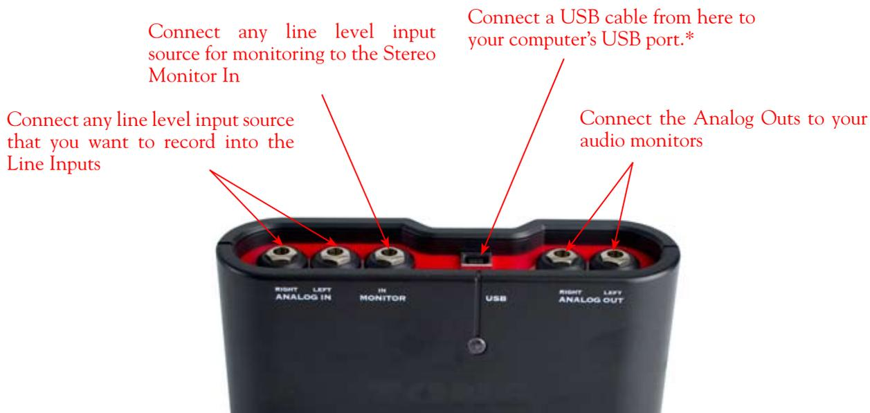
\*Note – be sure to always power off or mute your speakers or monitoring setup before connecting and disconnecting the USB cable between TonePort and your computer, as well as before booting up or shutting down your computer if TonePort is already connected. The best practice is to always power on your speakers last, and power them off first when connected to other audio gear to avoid a “pop”.
