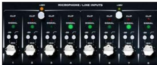
Rear panel XLR input levels are controlled by a row of trim knobs on the front panel. Use these inputs for microphones or balanced input signals with a gain range of 0 dB to 45 dB.
