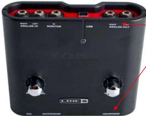
Connect the mono 1/4-inch Analog Line Outputs.
