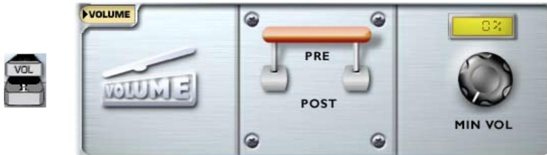
Vol (Volume) is one of GearBox’s Effects, and can be accessed remotely via an external MIDI controller device to provide you with a Volume pedal for your Gearbox “rig”. Note that the position of the Vol can be set “Pre” or “Post” in the signal chain.
