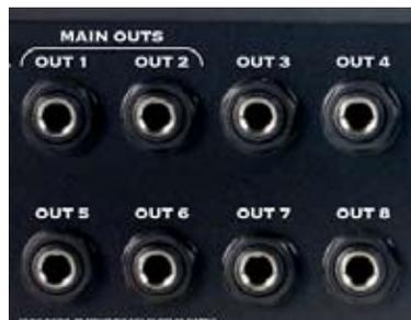
TonePort UX8 provides 8 balanced analog outputs (4 stereo pairs). For the cleanest audio signal, use 1/4-inch TRS cables to connect directly to your powered speakers, mixer or power amp setup.
