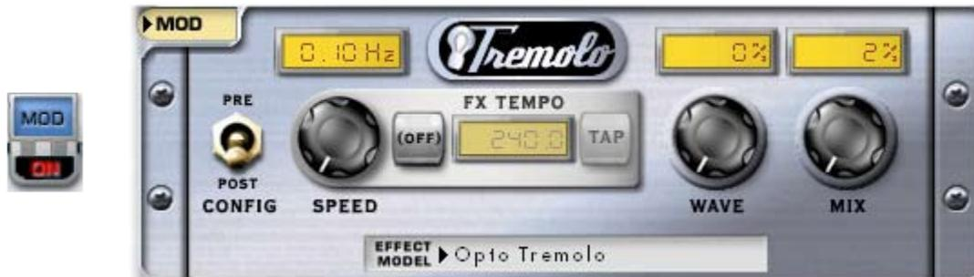
**Tremolo** is one kind of effect that can be run by GearBox’s **Mod** (Modulation) Effect. Tremolo produces a pulsing sound. It works by turning the volume of your input down and back up again repeatedly, at the speed set for the tremolo. For details on each of the Tremolo controls, move your mouse over the control and look in the Info Bar at the bottom of the GearBox window.
