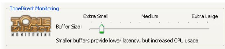
PODxt devices utilize a USB audio buffer (rather than ToneDirect™ Monitoring) which provides an independent, direct monitor signal with its own buffer adjustment. When a PODxt/Live/Pro is selected as the Line 6 device in this dialog, the ToneDirect™ Monitoring section of the dialog is replaced by a PODxt-specific “USB Audio Streaming” buffer slider:
