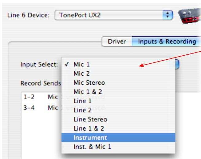
When GearBox is not in use, the Input Source Select menu is available. As shown here, TonePort devices offer several input Sources to choose from. The selected Source is what gets routed to the Device Sends.
