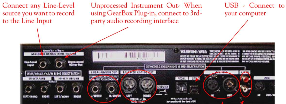
Analog Line Outs, Use either Unbalanced (1/4 -inch) jacks or Balanced (XLR) jacks to connect to your powered speakers or mixer
