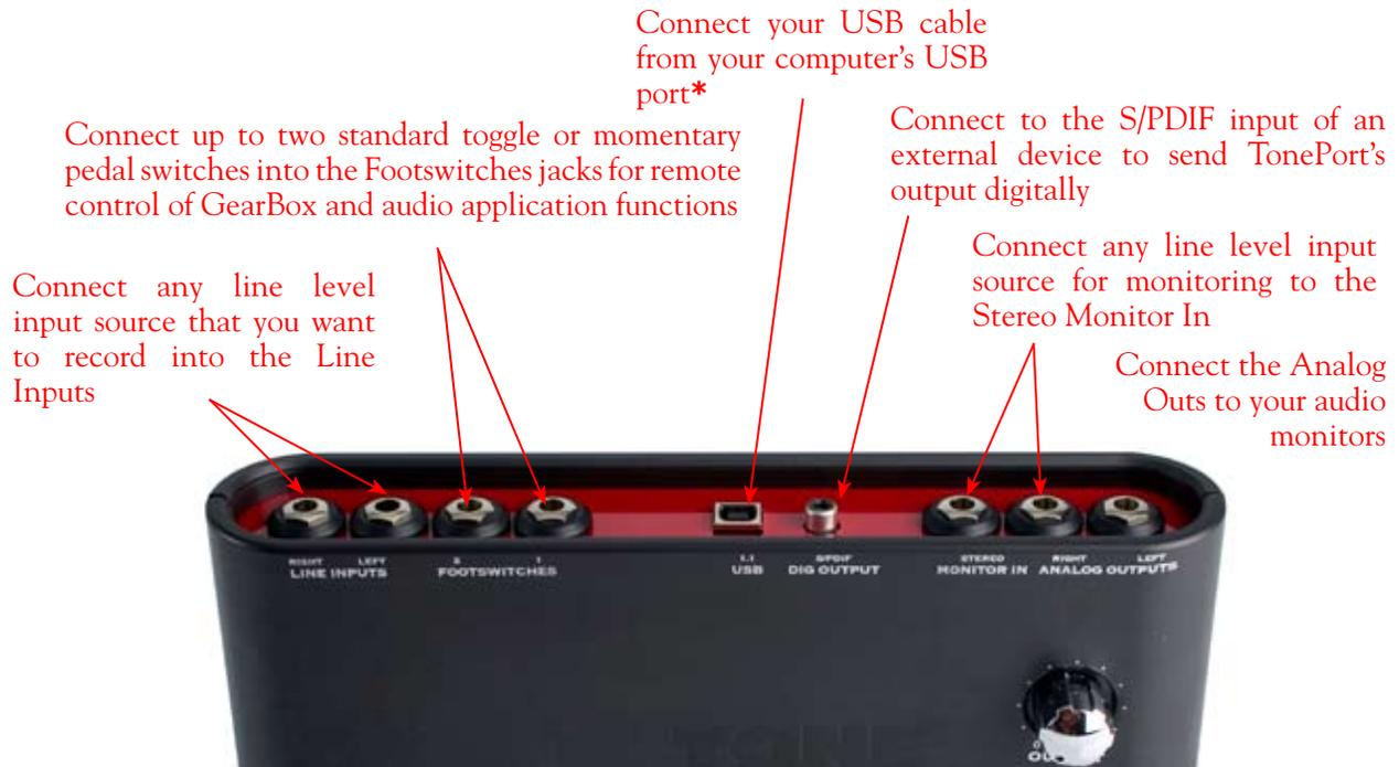
\*Note – be sure to always power off or mute your speakers or monitoring setup before connecting and disconnecting the USB cable between TonePort and your computer, as well as before booting up or shutting down your computer if TonePort is already connected. The best practice is to always power on your speakers last, and power them off first when connected to other audio gear to avoid a “pop”.
