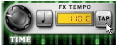
All GearBox’s Delay and Mod Effects (except for Rotary Drum + Horn) allow you to set their time/speed two ways. One way is to turn their speed or time knob. The other way is to choose a tempo.
