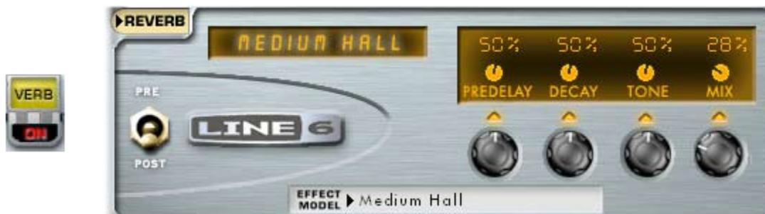
**Verb**, an abbreviation for **Reverb**, is one of the GearBox Effects. The Effect Model menu in the Reverb control panel lets you choose from a number of different models, including Spring Reverb as well as Room, Hall and Plate Reverb types:
