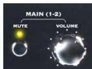
Main Outputs 1-2 are controlled by a main volume knob and main mute button. The volume knob is an analog level control and does not affect any level being sent to your computer. When Mute is engaged, as solid amber LED illuminates, blinking about once every 2 seconds.
