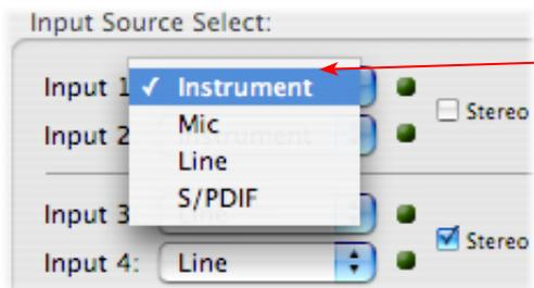
When GearBox is not in use, the Input 1 & input 2 selectors are available. As shown here, TonePort UX8 offers several input Sources to choose from. The selected Source is what gets routed to the Device Send.
