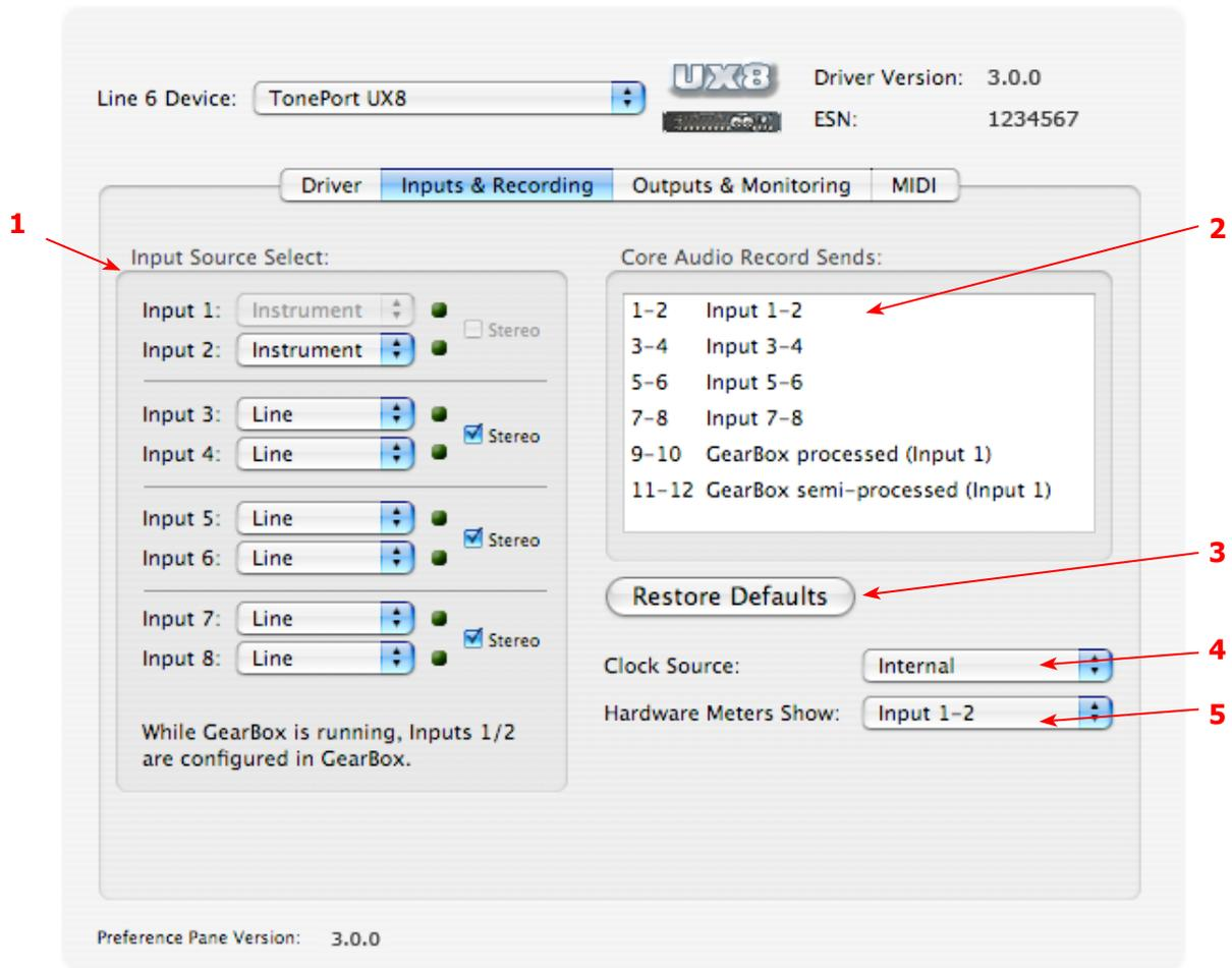
1 – **Input Source Select:** TonePort UX8 offers 8 individual input sources, each with its own selector where you can choose which physical input is to be used for each. Input source options are as follows:
