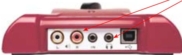
Connect a 1/8-inch stereo cord to the Headphone Out, or use the Stereo RCA Line outputs with an adapter.
