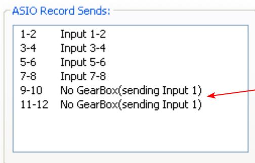
Sends 9-10 and 11-12 represent processed and semi-processed signals respectively, from the GearBox standalone application. If GearBox is not running, Sends 9-10 and 11-12 carry the signal from Input 1.
