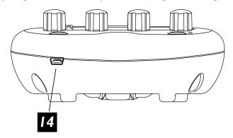
**USB** – You can connect Pocket POD to your Macintosh or Windows computer via the included USB cable and it'll automatically show up as a MIDI device. No drivers are needed!
