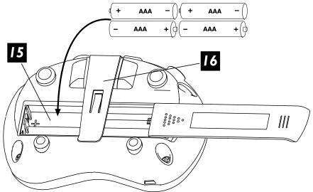
**Battery Compartment** – Pocket POD can run off (4) AAA batteries. To install them, slide off the battery door, insert the batteries in the orientation shown, then slide the battery door back on. Make sure you only use non-rechargeable alkaline batteries and dispose of them properly when they run out of juice.
