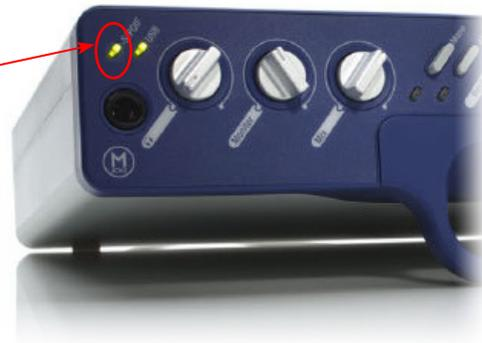
Note that when receiving S/PDIF input, the Input 1 & 2 level knobs on the front of the Mbox 2 do not adjust the digital signal level. To adjust the recording level, use the GearBox software's Tone volume and output level controls or your POD's S/PDIF Gain control.
