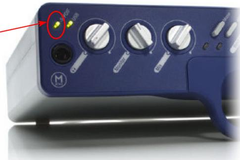
Note that when receiving S/PDIF input, the Input 1 & 2 level knobs on the front of the Mbox 2 do not adjust the digital signal level. To adjust the recording level, use the GearBox software's Tone volume and output level controls, or your PODxt or POD X3 S/PDIF Gain control.
