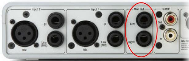
From the Mbox **Mon Out** jacks, connect to the Left and Right inputs for your powered speakers or monitoring system
