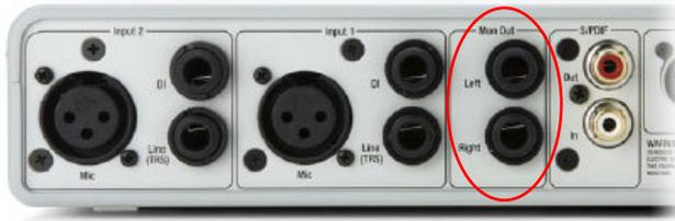
From the Mbox **Mon Out** jacks, connect to the Left and Right inputs for your powered speakers or monitoring system
