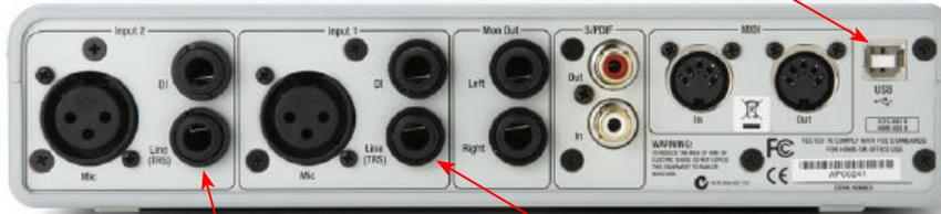
From your Line 6 device's **Right Analog Out** (or "Out 2"), connect to the Mbox 2 **Input 2 - Line input**
